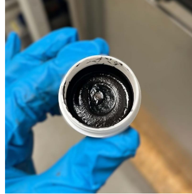
(b) MXene-Cu composite slurry after planetary mixing.
