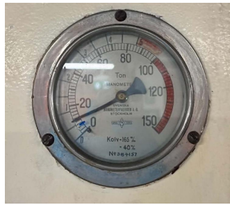
(b) Applied load of approximately 10 tonnes.
