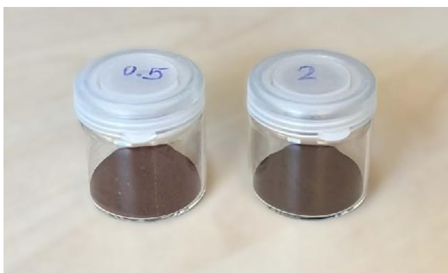
(a) Freeze-dried MXene-Cu composite powder.
