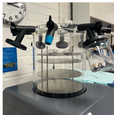
(b) Freeze-dryer used to remove the frozen solvent by sublimation.
