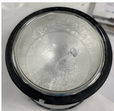
(a) Composite mixture in an Eppendorf tube during freezing in liquid nitrogen.
