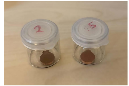
(c) Pressed composite samples after cold pressing.
