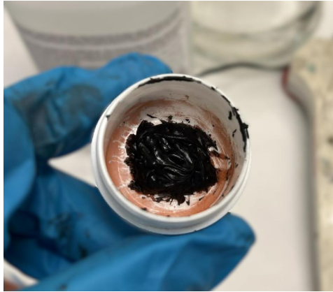
Figure 3.1: Premixed MXene-Cu composite slurry. Mixed with a needle.
