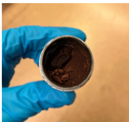
(b) A combination of compact MXene-Cu composites and MXene-Cu composite powder after freeze-drying.
