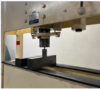
(a) Hydraulic press setup used for cold pressing.
