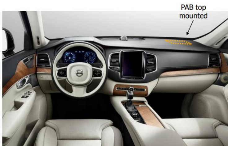
Figure 3 Passenger airbag front side installed in the car's dashboard
