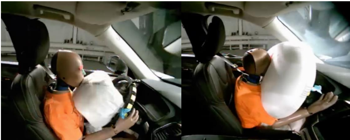
Figure 6 Driver's airbag fully deployed (Euroncap, 2022)
