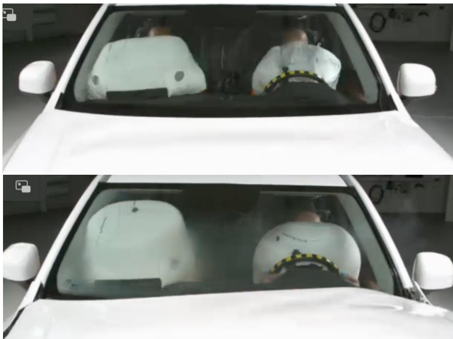
Figure 7 Passenger and driver's airbag fully deployed (Euroncap, 2022)
