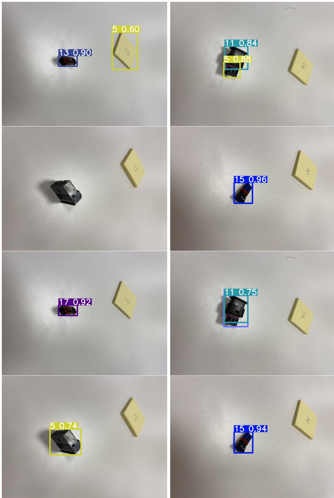
Figure 4.12: The upper four images show the results of YOLOv5 trained on Clean Dataset, tested on the real dataset. The lower four images show the results of YOLOv5 trained on Distract Dataset, tested on the real dataset.
