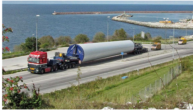
Figure 2.1: Example of a transport of a part of a conventional wind turbine tower
