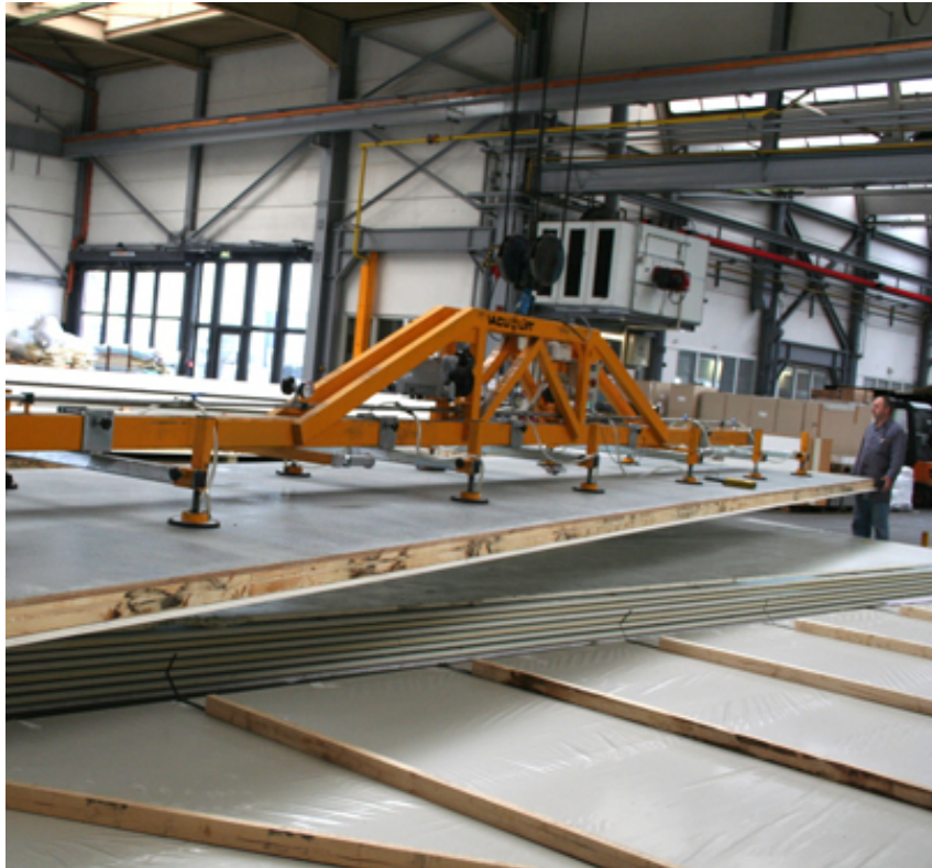
Figure 4.9: An example of a traverse equipped with a suction cup [43]
