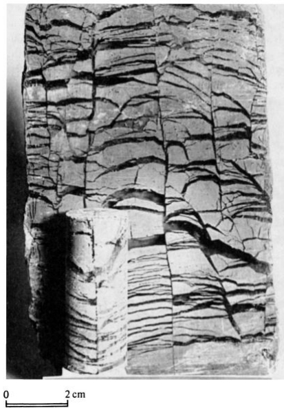
Figure 2.3: Frozen soil experiencing frost heave, showing ice-lenses/bands (Williams & Smith, 1989)
