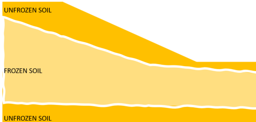
Figure 2.2: The potential stratification of a thawing slope, authors own illustration.
