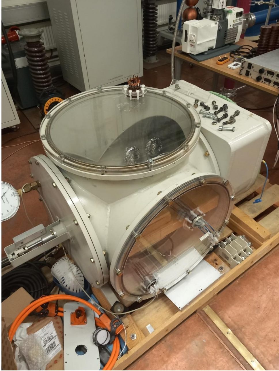
Figure 9: The vacuum chamber photograph
