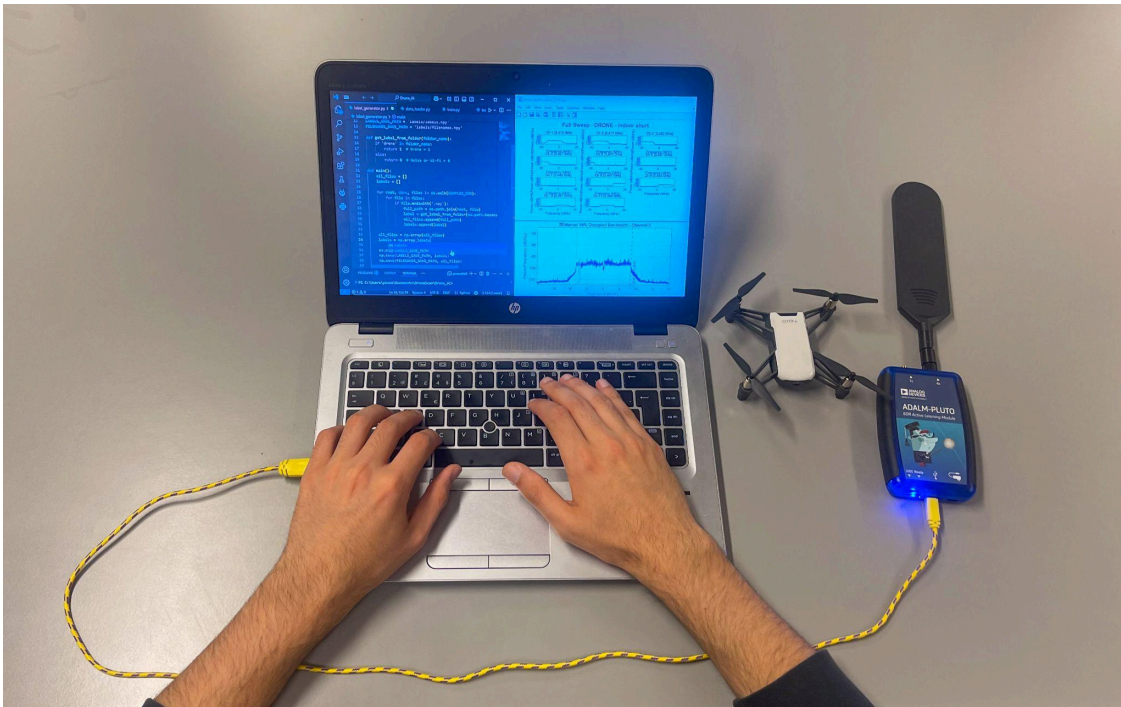
Fig. 8. Hardware setup including Windows laptop, ADALM-PLUTO SDR with 18 dBi paddle antenna, and Ryze Tello drone.
