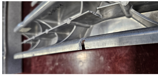
(a) Visible damage from ejector pins
