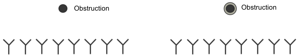
Figure 1.1: Top view schematic of the situations to be analyzed, e.g. an obstruction without or with material coverage in the vicinity of an array antenna.
