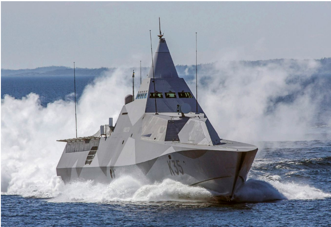
Figure 1.2: Visualization of cords/poles mounted on a ship such that an antenna's view will be obstructed. The image shows Saab AB's Visby-Class Corvette K35 [6].
