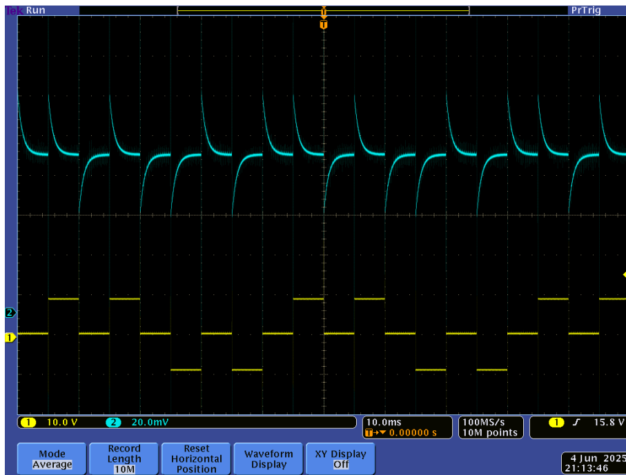
Figure 4.14: DUT current in relation to the three-level voltage waveform.
