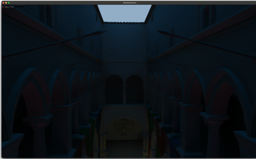
Figure 6.4: The Sponza model with 3 emissive hornbug models by McGuire [10] showcasing off-screen indirect light coming from a pink, blue and a yellow hornbug.
