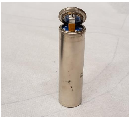
Figure 20 After circular cut
