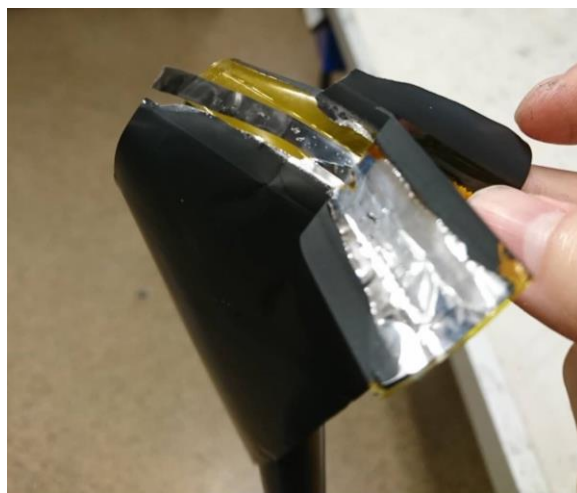
Figure 36 The cathode lead is located in between the cathode foil
