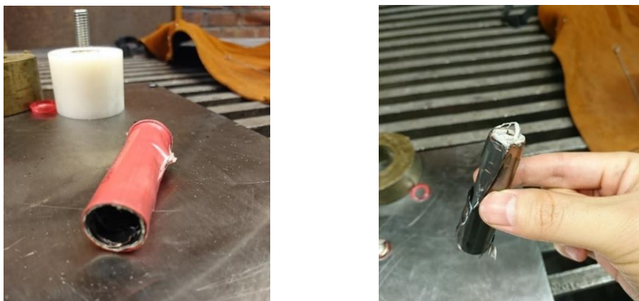
Figure 9 a) The housing with plastic shell (left), b) The cell (right)
