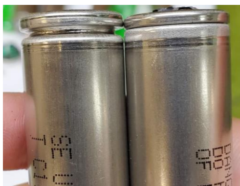
Figure 10 Different safety vent designs
