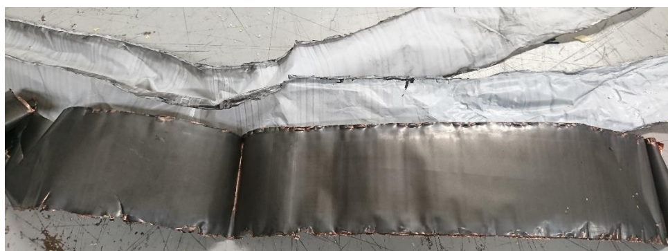
Figure 37 Anode foil and separators in the ordinary case
