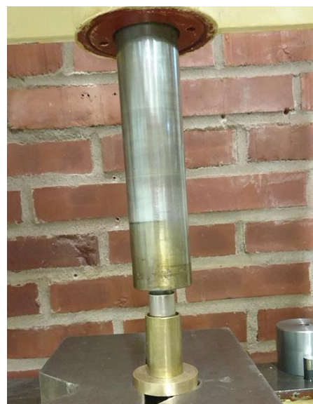
Figure 26 a) 500kg for pushing the 16mm pusher, b) The front view of the hydraulic press in the push step
