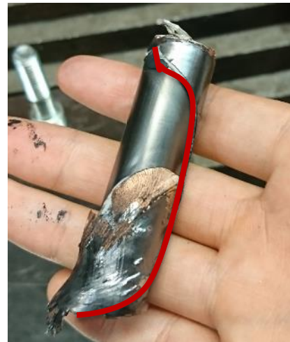
Figure 25 a) 16mm pusher, b) The uneven edge is marked in red
