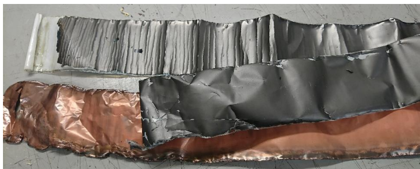
Figure 34 An example of an aging battery
