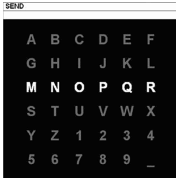
Figure 2.1: A typical P300 speller grid with the middle row highlighted [1].
