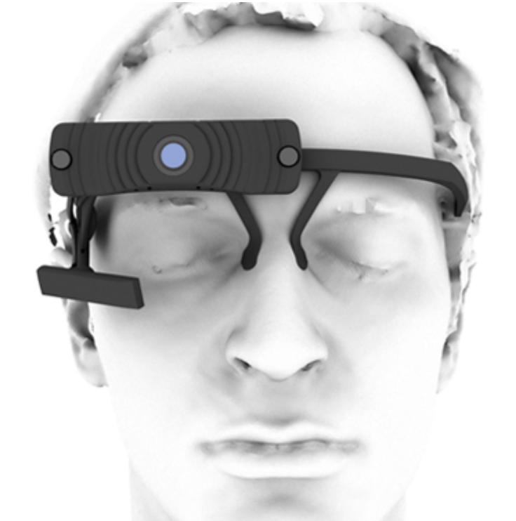
Figure 4.5: A rendering of the Pupil Labs eye tracker with one eye camera tracking the right pupil. The front-facing world view camera is visible at the top. From the Pupil Labs store [5].
