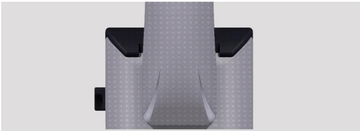
Figure 27 - Detailed view of the split lines at the lower part of the handle. Authors' own figure.
