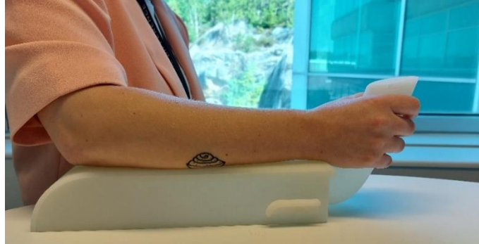
Figure 22 - The 3D printed joystick concept shown in use that were evaluated during the workshop. Authors' own figure.
