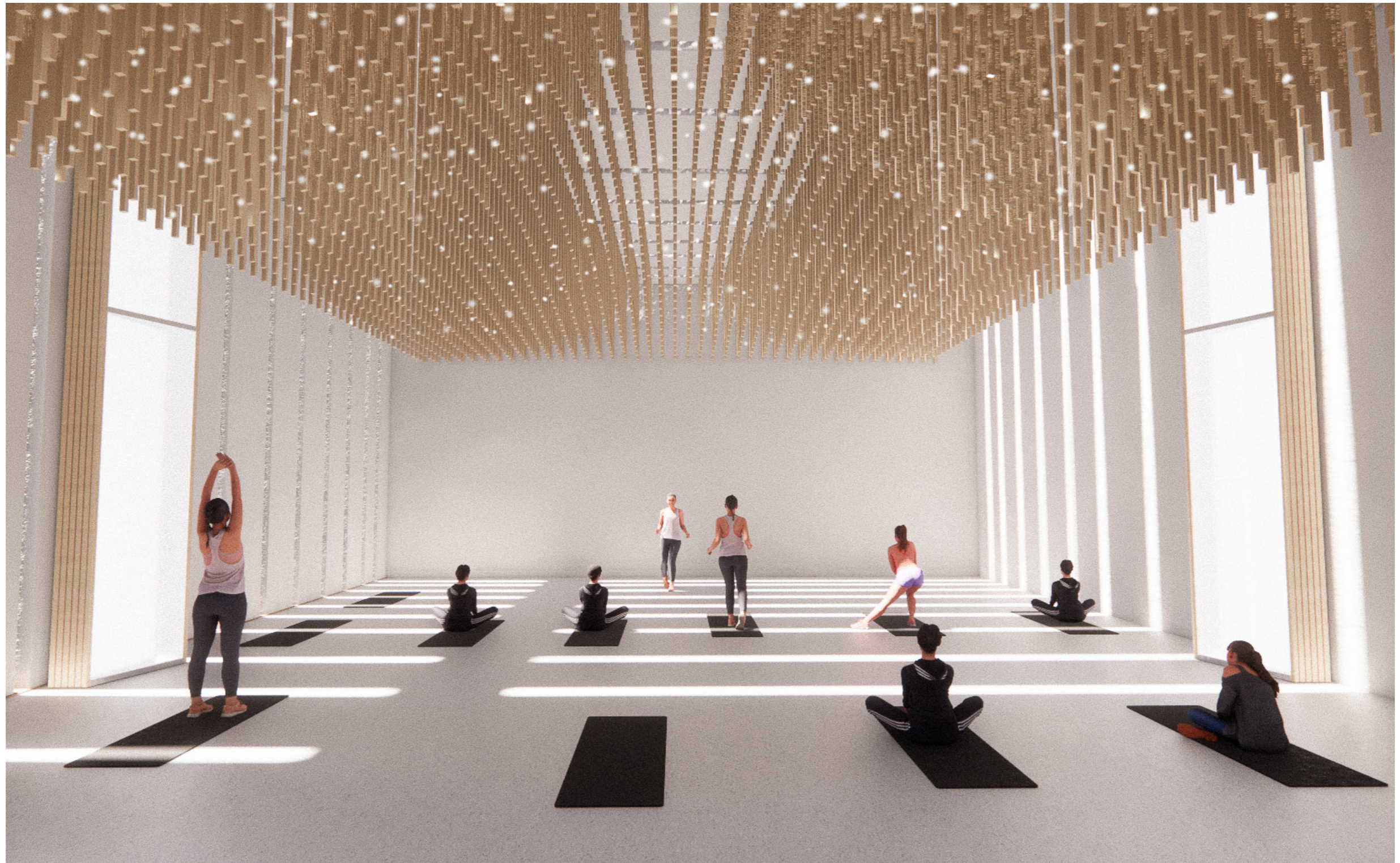
View of the group lesson hall, seen from the entrance. The cuts in the wall are making a dynamic expression on the floors and the wall that will change through the day. The lights in the roof are meant to create the same effect but in artificial form - this to ensure that the room doesn't lose its qualities completely during cloudy days or in the darker winter months.
