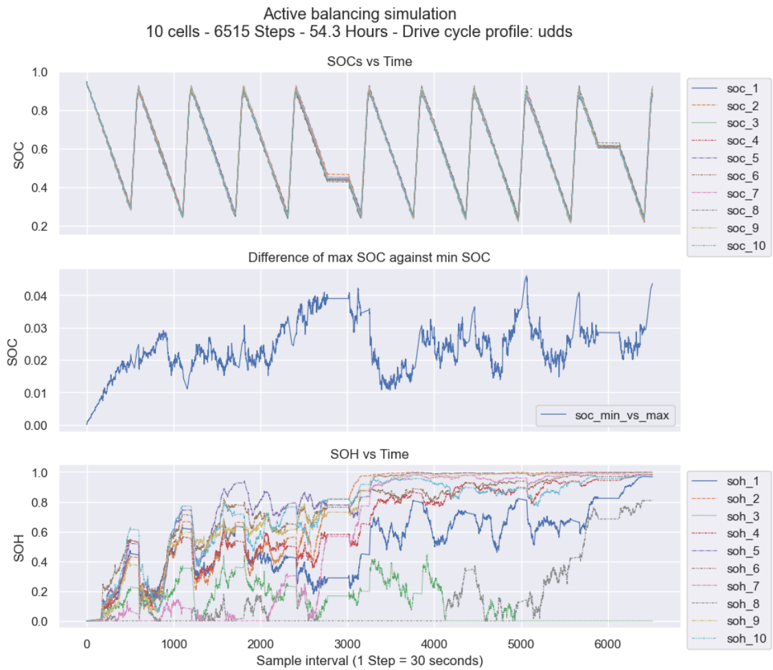
Figure 4.9: Active balancing for SOC and SOH - 1% threshold - case 3.
