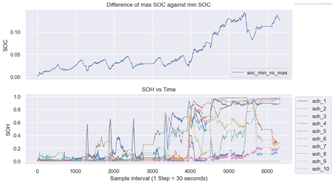
Figure 4.13: Active balancing for SOC and SOH - 3.5% threshold - case 1.
