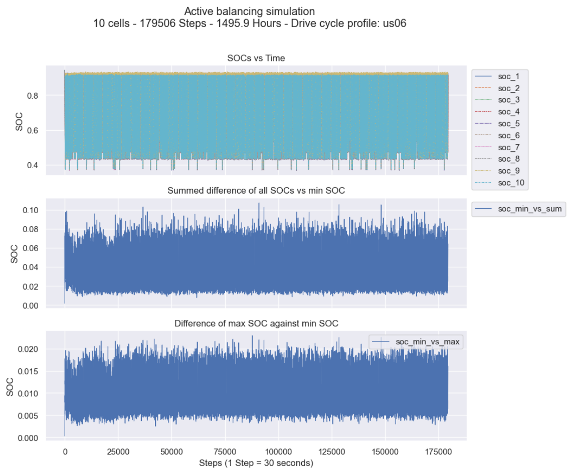
Figure A.2: Active SOC balancing test - 1000 cycles - utilization [20, 2].
