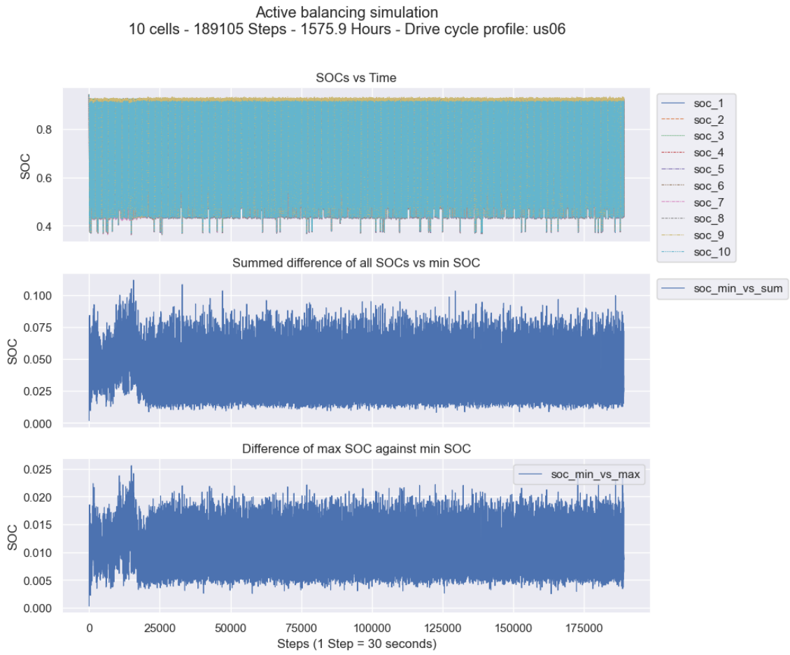
Figure A.1: Active SOC balancing test - 1000 cycles - utilization [10, 2].
