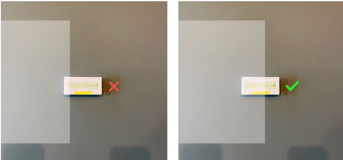
Figure 7.1: Demonstration of the visual affordance for light edge alignment when using automatic edge detection. Left: Not properly aligned. Right: Properly aligned.
