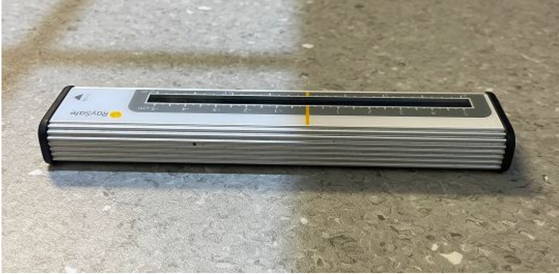
Figure 3.1: A DXR+ positioned with its designated yellow line at the light field edge. The light field edge fades out with a so-called penumbra. In this case, the DXR+ is positioned at the end of the penumbra.
