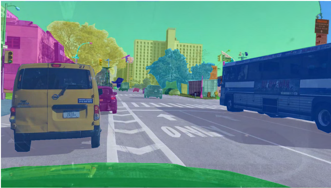
Figure 1.1: The above figure is taken from the BDD100K dataset that is made available by Berkeley University. On the figure we can see a full-frame segmentation of a road with automotive vehicles.
