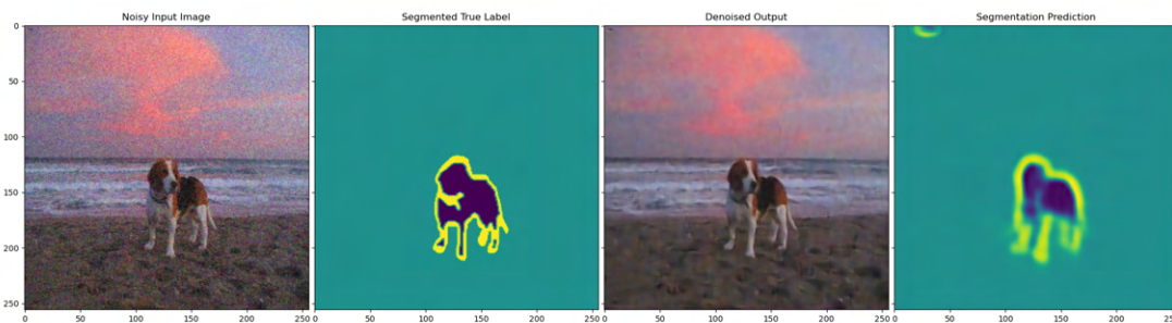
Figure 4.7: The figure shows a slight incorrect segmentation result from the dog class. There is a soft artifact on the top and at the same time the outline seems a bit blurred, which might be hard to miss by binarizing the image.
