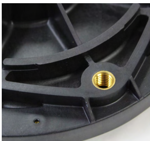
Figure 2.10: Embedded metal compression limiter
