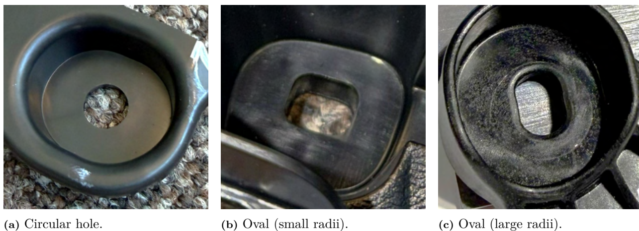
Figure 4.42: Comparison of the characteristic clearance hole geometries present in the tested thermoplastic components.
