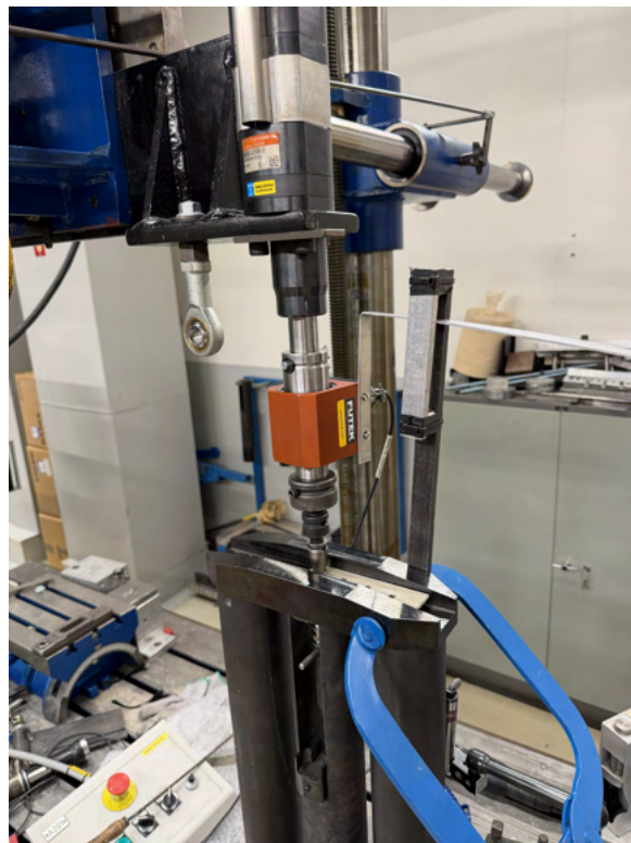
Figure 3.6: Experimental rig utilized for friction and preload relaxation characterization.
