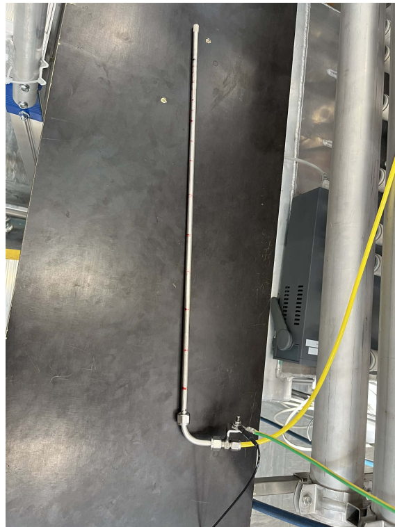
Figure A.5: The CO_2 measuring probe with markings at 0, 12, 21, 36, 48, 62, 78, 93, 121, 150, 200, 255, 306, 358, 411 and 460 mm.
