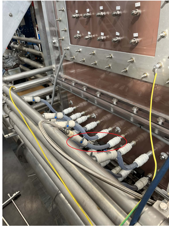
Figure A.4: Point of injection with added plug for reduction of cross-sectional area.
