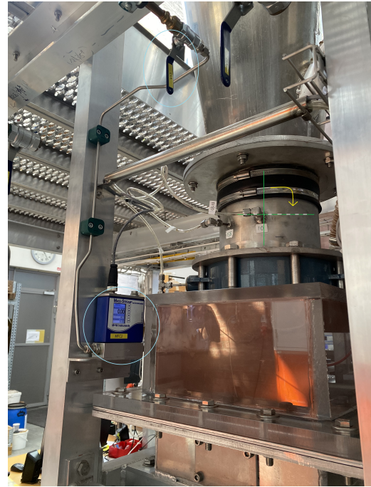
(b) Exit of cyclone with schematic picture of the butterfly-valve operation.
