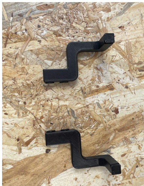
Figure 17. 3D-printed gripper claws adapted for PCB handling.
