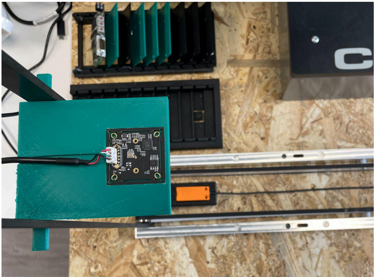
Figure 9. Camera mount and top-down view of the conveyor showing the visual field and pickup zone
