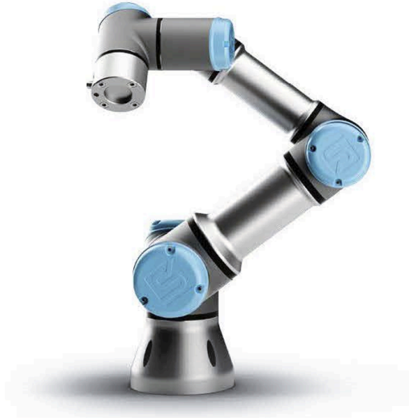
Figure 1. The UR3 collaborative robot from Universal Robots. The image shows the robot's compact form factor and six joint configuration. Source: Universal Robots (2016).
