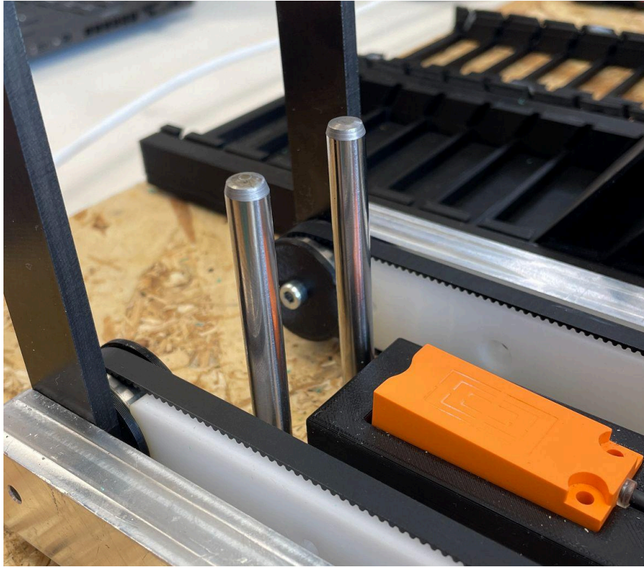
Figure 14. Fixed positioning pins at the conveyor end used to align PCBs prior to gripping.
