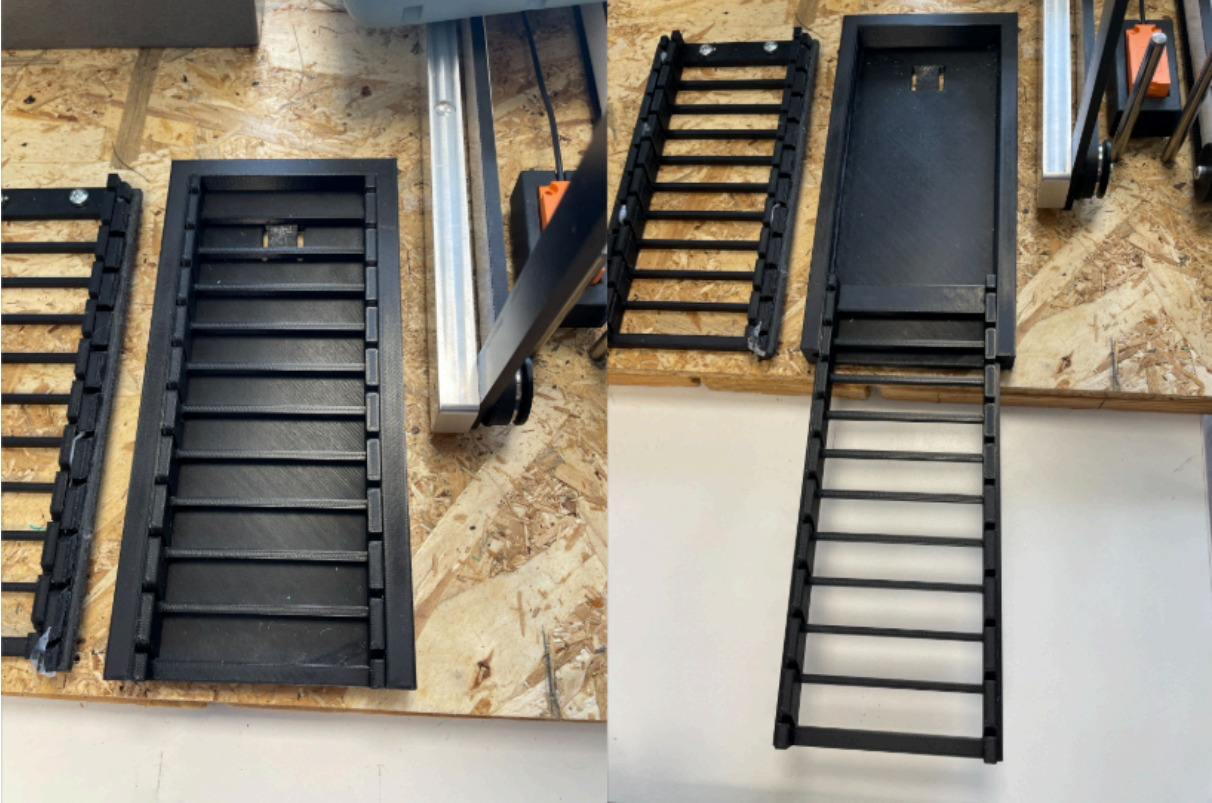
Figure 15. Two-part 3D-printed tray system with removable insert for full board collection.
