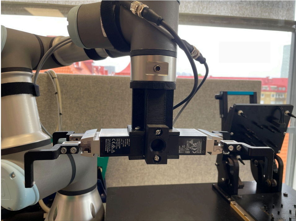
Figure 12. Dual gripper mount with 3D-printed claws for alternating PCB pick and place.
