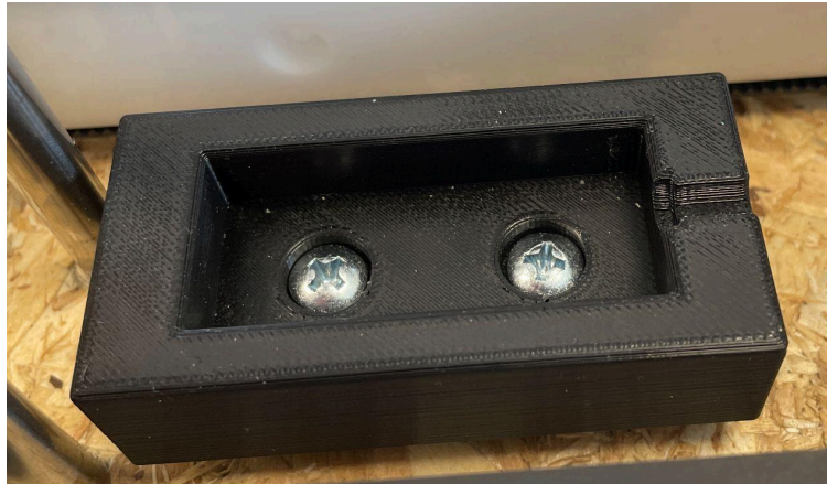
Figure 18. 3D-printed housing for capacitive sensor, mounted between the conveyor rails.
