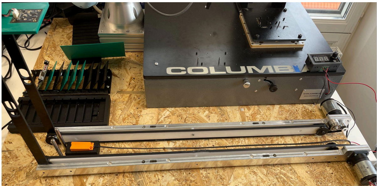
Figure 11. Final conveyor with timing belt and toothed drive wheels.
