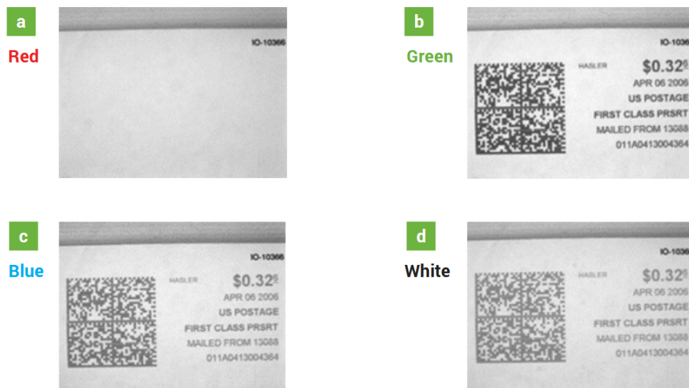
Figure 2.8: Different wavelengths of illumination used on a paper-stamp with red-text [28].
