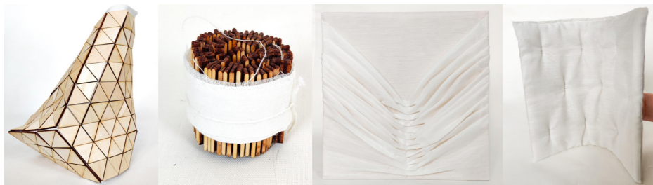
On top These four are less merged than the other. In two of the examples, Triangles and Rollup, the wood and textiles are glued together and the other two, Ruching and Soft wood, The wood is sewn in to the textile.
