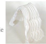
Pleated vault This is the most flexible due to the fact that there is no wood added yet.
