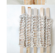
Wood weave, Wood knit and Roll up is quite similar. They are flexible in the direction of textiles but stiff in the direction of the wood. They are ordered in the order of which has the most flexibility in the textile.
