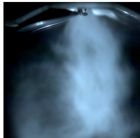
(d) Instantaneous picture of spray with 100 bar injection pressure 264.2 CAD before TDCF.
