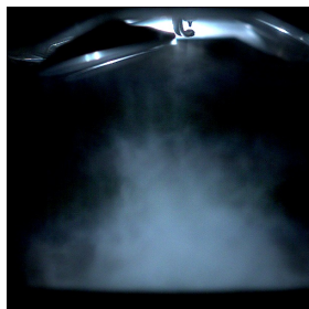
(h) Instantaneous picture of spray with 200 bar injection pressure 269.7 CAD before TDCF.
