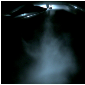
(j) Instantaneous picture of spray with 100 bar injection pressure 266.5 CAD before TDCF.
