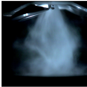
(d) Instantaneous picture of spray with 100 bar injection pressure 276.1 CAD before TDCF.
