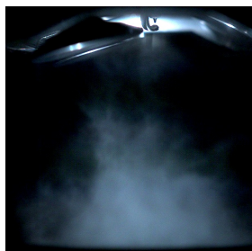
(k) Instantaneous picture of spray with 200 bar injection pressure 266.5 CAD before TDCF.
