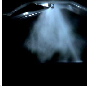
(a) Instantaneous picture of spray with 100 bar injection pressure 287.3 CAD before TDCF.
