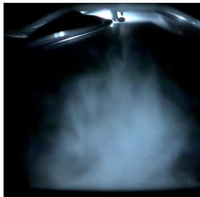
(g) Instantaneous picture of spray with 100 bar injection pressure 269.7 CAD before TDCF.
