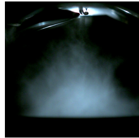
(f) Instantaneous picture of spray with 350 bar injection pressure 276.1 CAD before TDCF.
