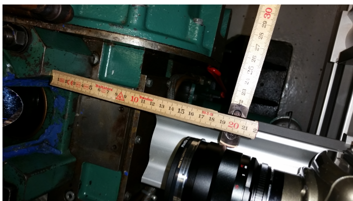
Figure 3.3: The pictures shows the distance between the camera and the engine in under view mode.
