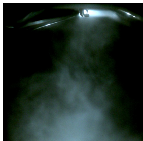
(h) Instantaneous picture of spray with 200 bar injection pressure 248.3 CAD before TDCF.
