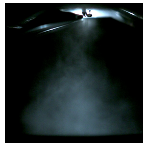
(i) Instantaneous picture of spray with 350 bar injection pressure 269.7 CAD before TDCF.
