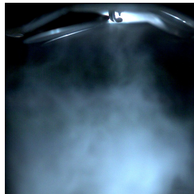
(e) Instantaneous picture of spray with 200 bar injection pressure 264.2 CAD before TDCF.
