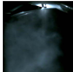
(f) Instantaneous picture of spray with 350 bar injection pressure 264.2 CAD before TDCF.
