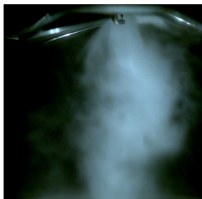
(g) Instantaneous picture of spray with 100 bar injection pressure 248.3 CAD before TDCF.
