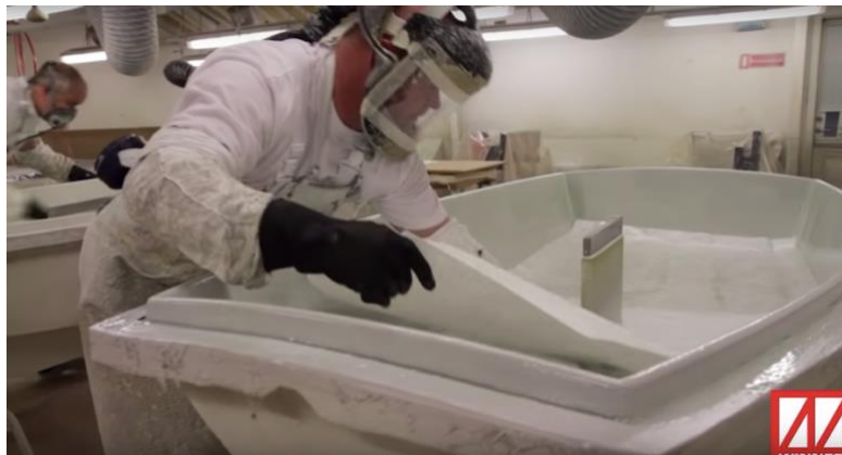
Figure 16. Applying reinforcement to the mold, (Martinfruergaard, 2012).
