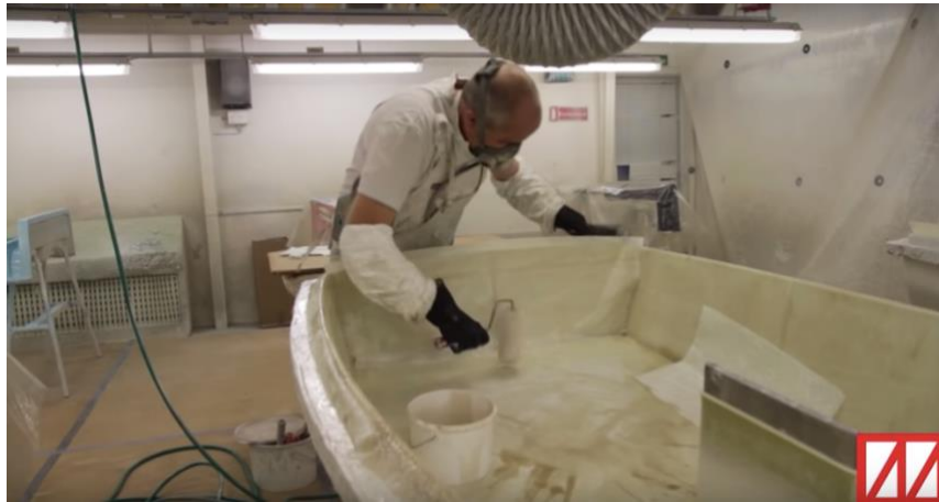
Figure 17. Manual lamination process, (Martinfruergaard, 2012).
