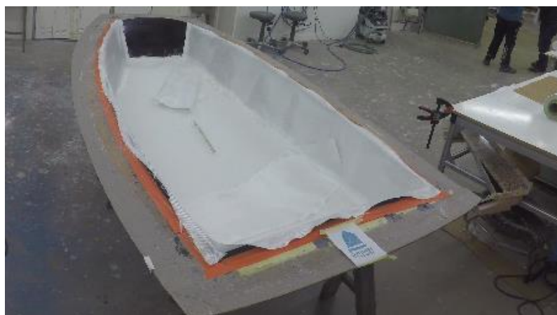
Figure 7. Apply reinforcement (glass fiber roving).
