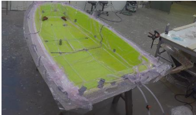
Figure 12. Vacuuming mold together with reinforcement.
