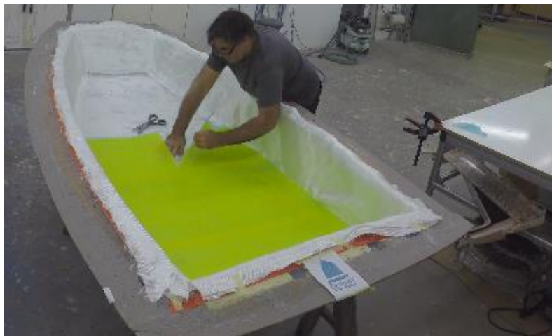
Figure 9. Applying resin transport medium.
