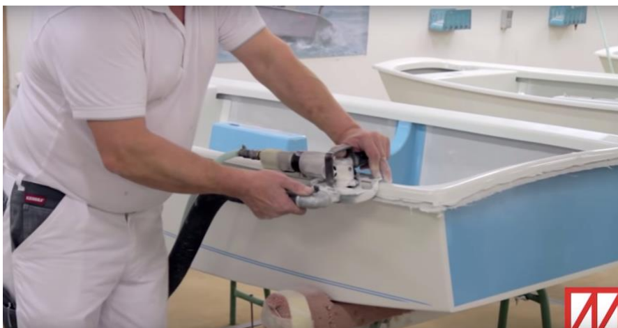
Figure 21. Grinding and polishing, (Martinfruergaard, 2012).
