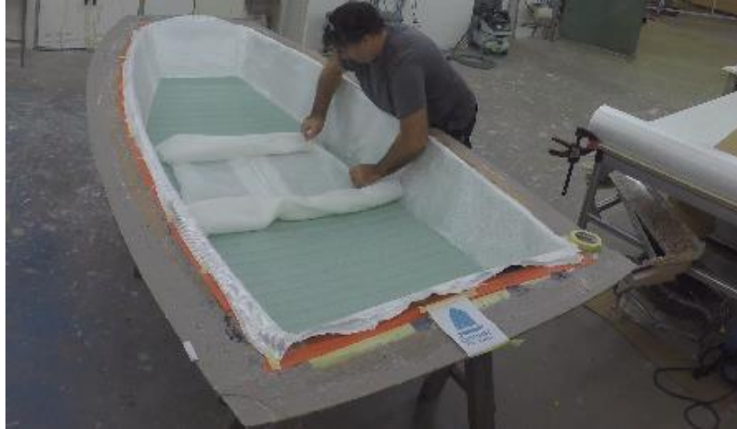
Figure 8. Applying reinforcement (PET foam core and surface mat).
