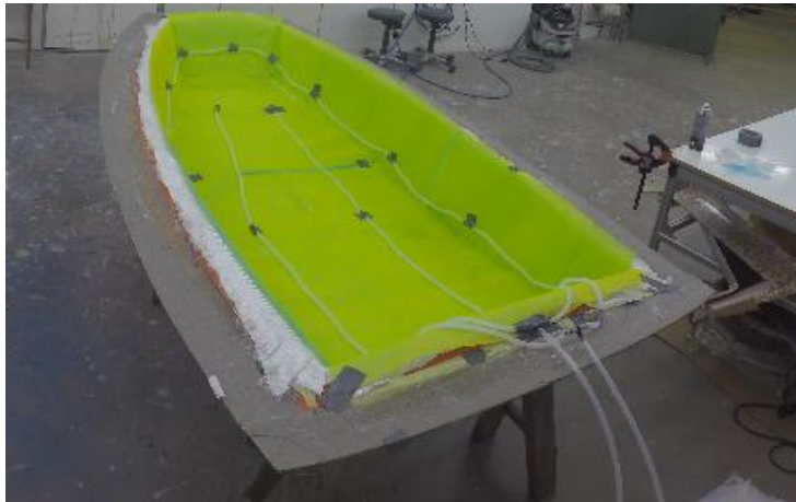
Figure 10. Design and installation of resin feeding/vacuum lines.
