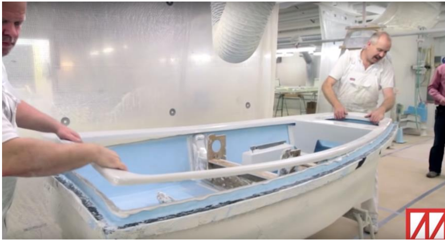
Figure 19. Gluing parts together, (Martinfruergaard, 2012).
