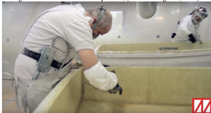
Figure 18. Laminating the corners/seams, (Martinfruergaard, 2012).
