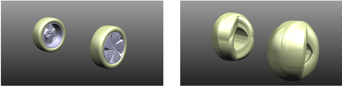
Figure 6.13: The 3D geometry of the wheel to the left, compared to the motion envelope of the wheel to the right.
