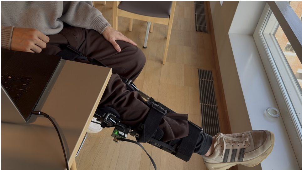
Figure 4.15: Experimental setup for synchronization validation during cyclic knee motion.
