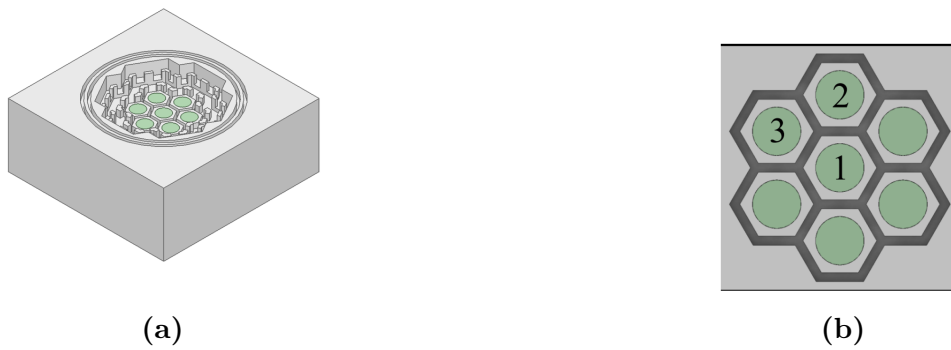
Figure 4.1: Focal Plane Array designed and optimized for 94GHz:(a)FPA Lateral view (b)Top View [4]
