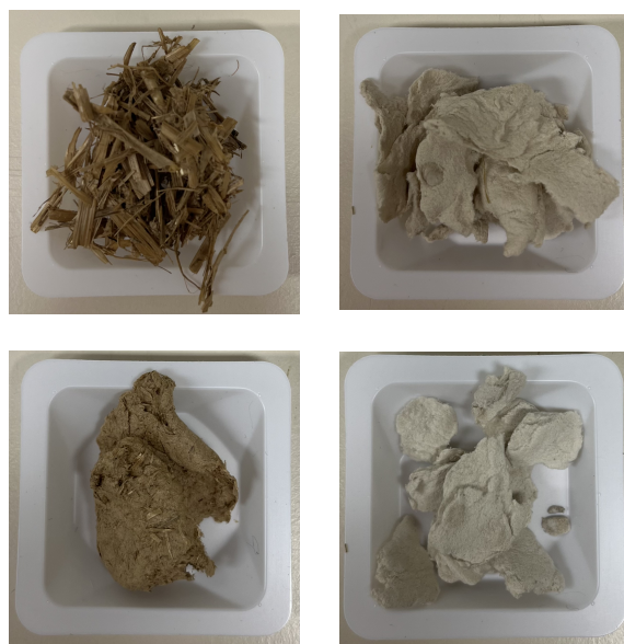
Figure 4.4: Top row: pretreatment of cellulose without acid (left) and soda pulping (right). Bottom row: pretreatment with acid (left) and soda pulping (right)
