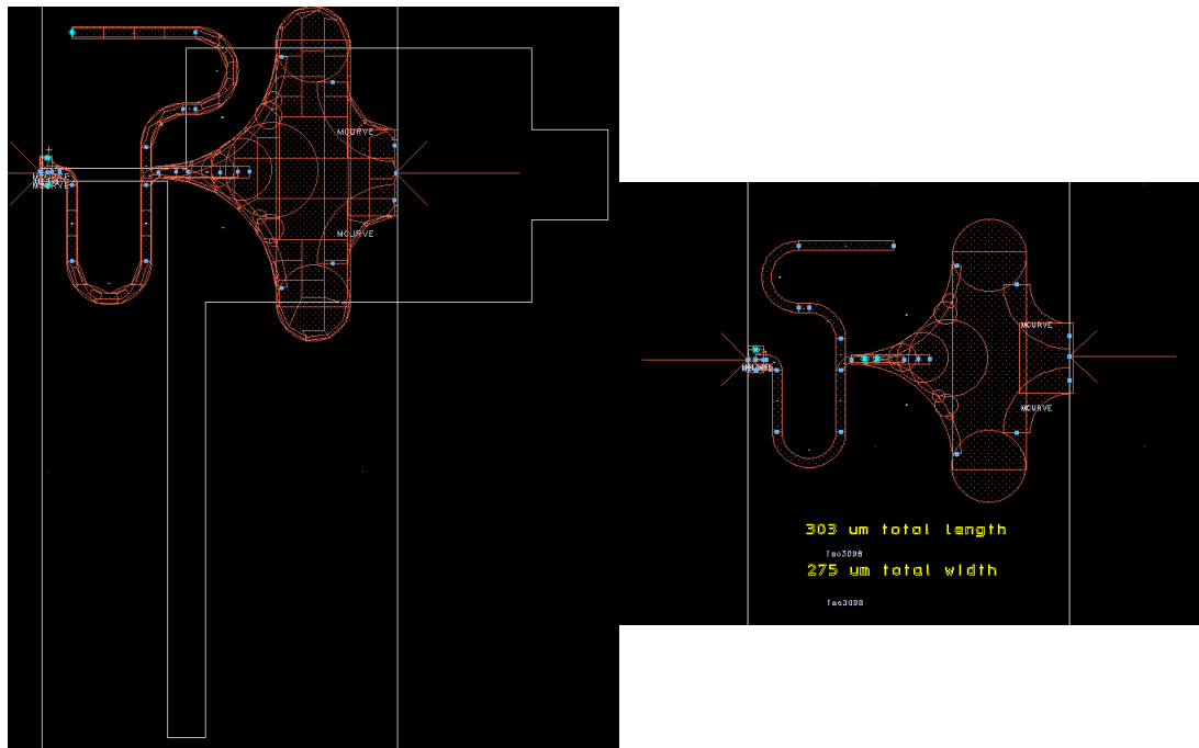
Figure 44. New matching network on chip side. To the left the size difference from Silvia’s design. The old matching network is in white lines.
