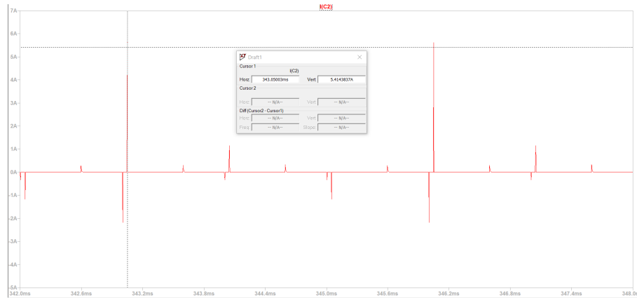
Figure 3.2: The overshoot of the current due to the winding sample
