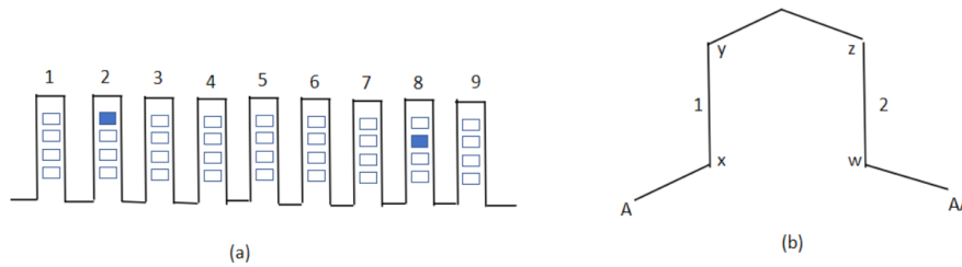
Figure 2.14: The first turn has active sides in first and second layers [12]
