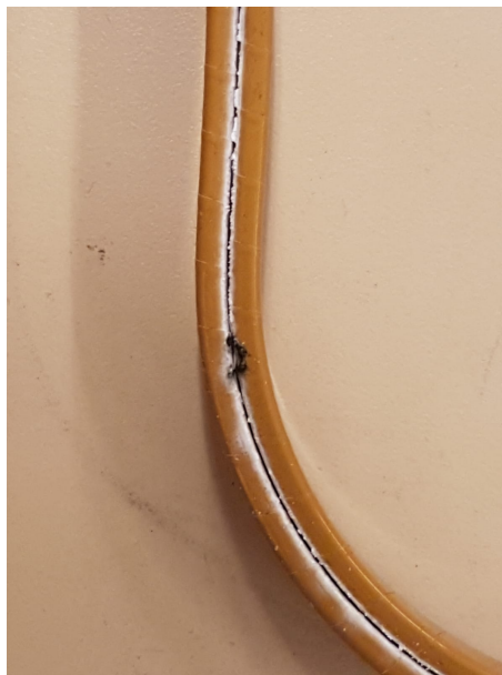
Figure 5.6: The failure of ECRC67 sample
