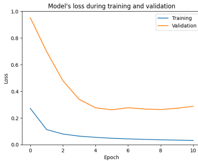
Figure 4.5: Training and validation progress of the CNN model with four residual blocks and a dropout rate of 0.
