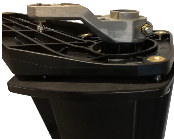
Figure 14: Steering shaft (Note that it is upside down compared to when inside the WR)
