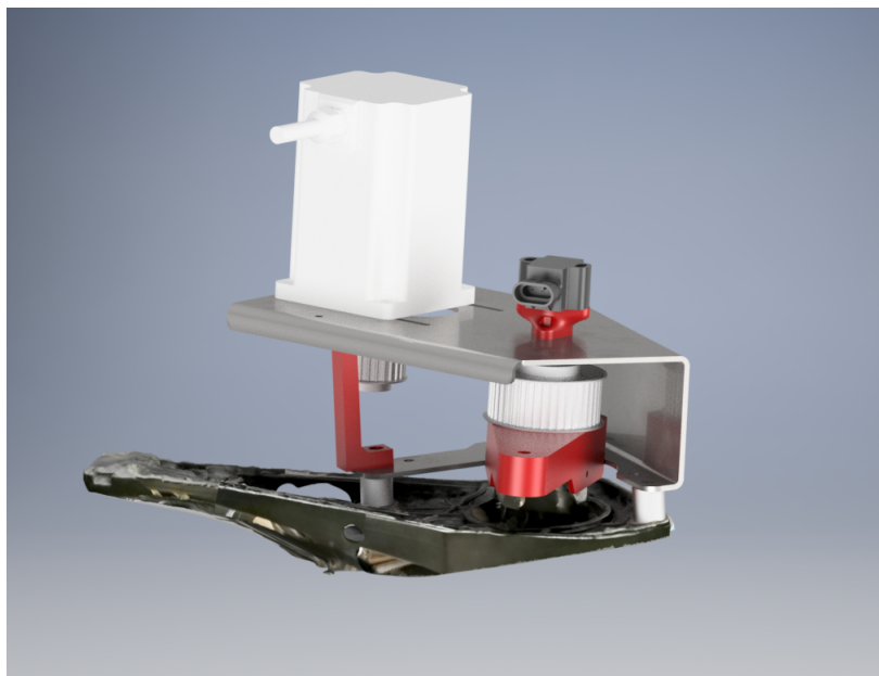
Figure 21: The complete construction for mounting the motor, pulleys and angle sensor
