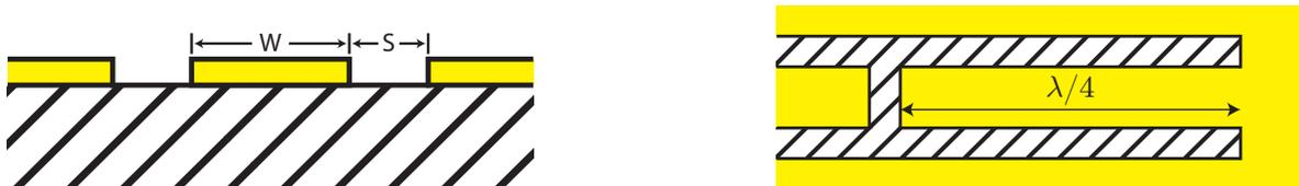
Figure 2.1: *Cross-section (left) and top view (right) of a quarter wavelength coplanar waveguide with the centre conductor and ground plane (yellow) on top of a substrate (hashed). The centre conductor of width  $W$  is separated from the ground plane by gaps of width  $S$ . The resonator is terminated by an open end on one side and a shorted end on the other.*
