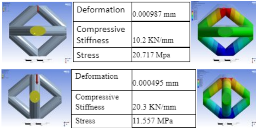
Figure 4.9: Compressive stiffness of diamond lattice geometry for x direction load and z direction load respectively
