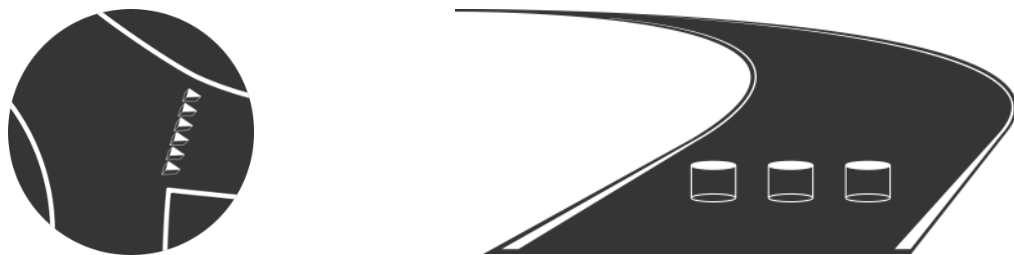
Figure 31 Illusion that prevents wrong turn in intersections (left) and illusion that stops the WW-drivers in the middle of an entrance/exit ramp (right).
