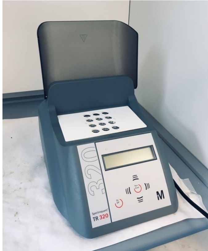
Figure 3.2. Heat block used in the COD analysis.
