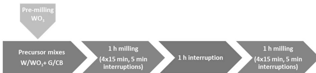
Figure 3: Schematic of the ball milling sequence. Interruptions of milling were done in order to reduce the input of thermal energy. Pre-milling, solely of the \text{WO}_3 precursor powders was performed at the same conditions and following the same sequence as the precursor mixes.
