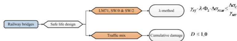
Figure 2.11 Fatigue design procedure of railway bridges
