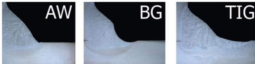
Figure 2.3: Weld toe in AW, BG and TIG dressed state, from Shams-Hakimi et al., 2015.
