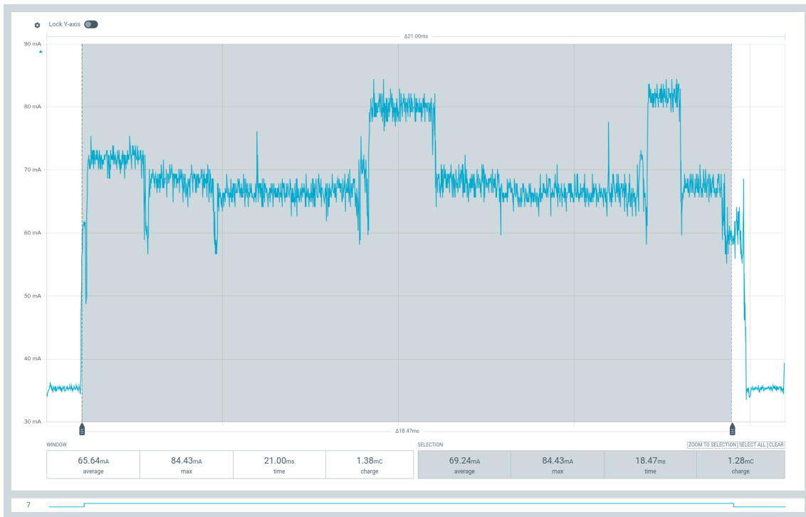
Figure D.4: Power profile of the Pareto-optimal HR Standalone mini_1ch model utilizing the realistic FLASH+SRAM deployment configuration. Due to aggressive structural pruning, the model fits almost entirely within the ESP32-S3’s cache, allowing it to complete inference in 21 ms with minimal external bus penalty.
