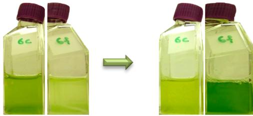
Figure 5: Left: *C. protothecoides* on day 4 in municipal wastewater (6c, left) and artificial growth medium (6f, right). Right: Same cultures on day 22. Growth in the artificial growth medium (6f, right) was slower than in the wastewaters (6c, left).
