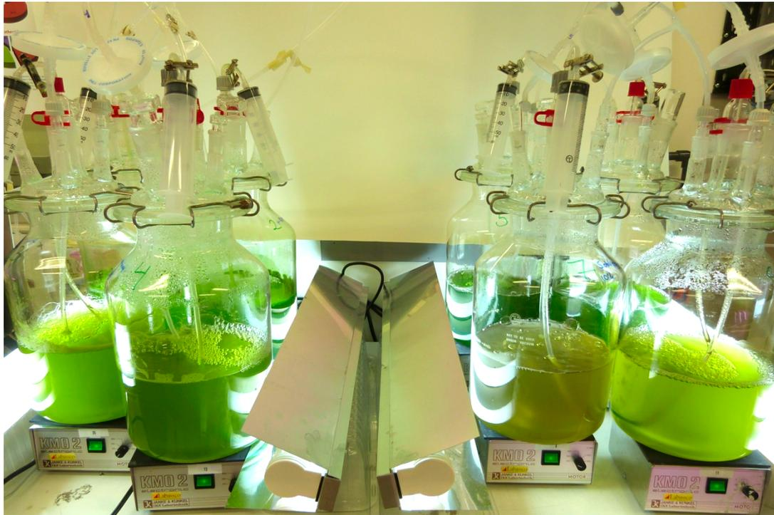
Figure 3: Algae cultivation setup. To the left are the four cultures of *D. pulchellum* and to the right *S. obliquus*.
