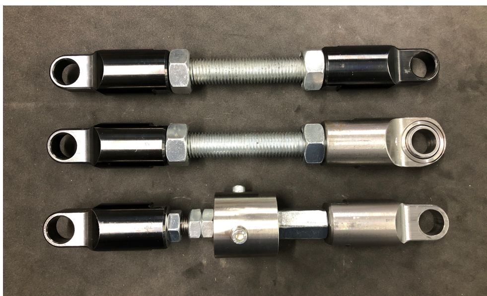
Figure 63 The three shock dummies used in the first angular force test rounds.
