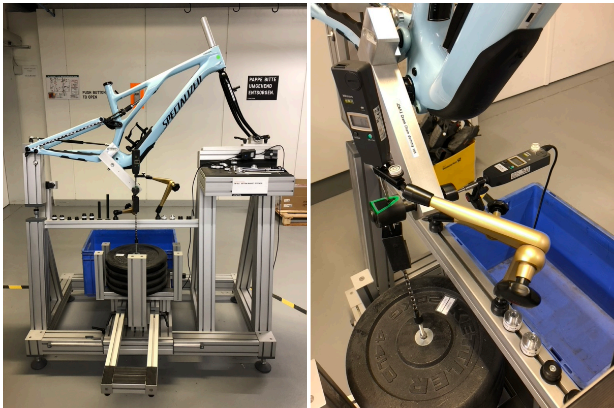
Figure 23 Zedler's Bottom Bracket Stiffness test bench and set up with a full suspension mountain bike frame
