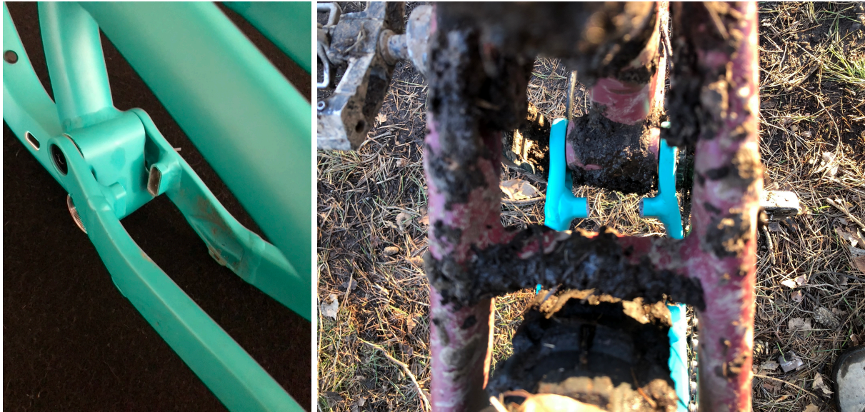
Figure 6 A rear triangle made less stiff through cutting off the bridge in between the chain stays.
