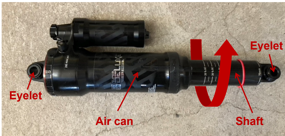
Figure 36 The main parts of a mountain bike rear shock.
