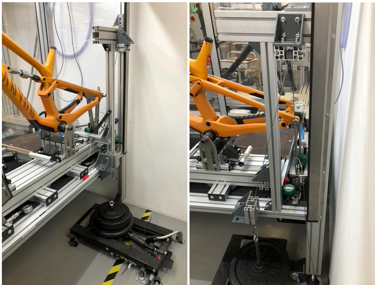
Figure 61 The initial set up of the angled force test.
