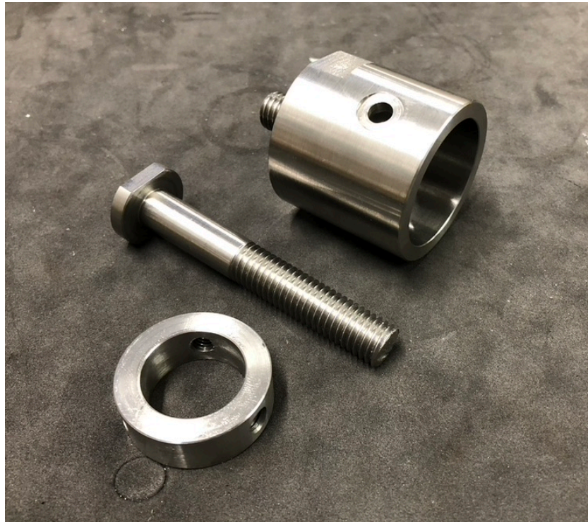
Figure 40 Parts machined for the rotating shock dummy.
