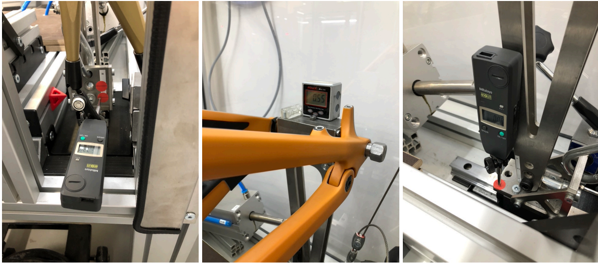
Figure 66 New locations for the measuring devices in the second test iteration.
