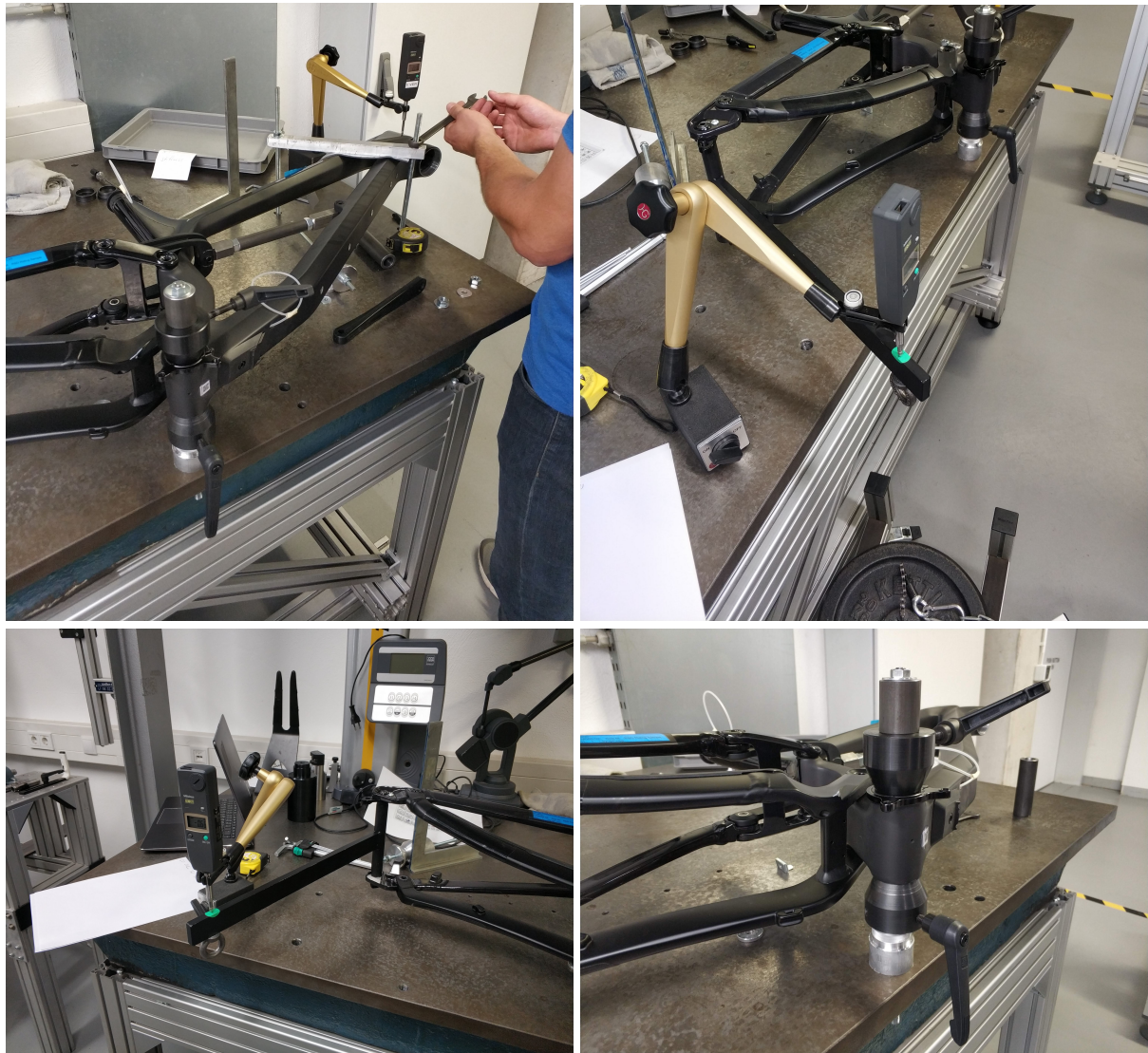
Figure 27 Test of conceptual test rig for measuring rear triangle stiffness. Reproduced with permission.
