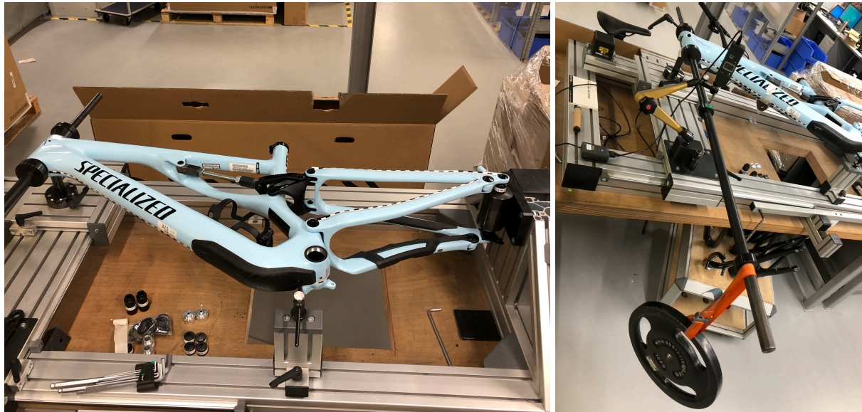
Figure 21 Zedler's head tube stiffness test performed in the manufacturers test lab.
