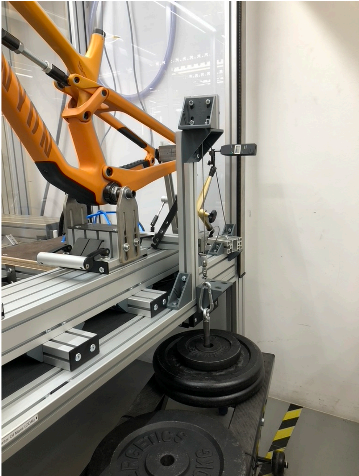
Figure 72 Test setup for the horizontal force.
