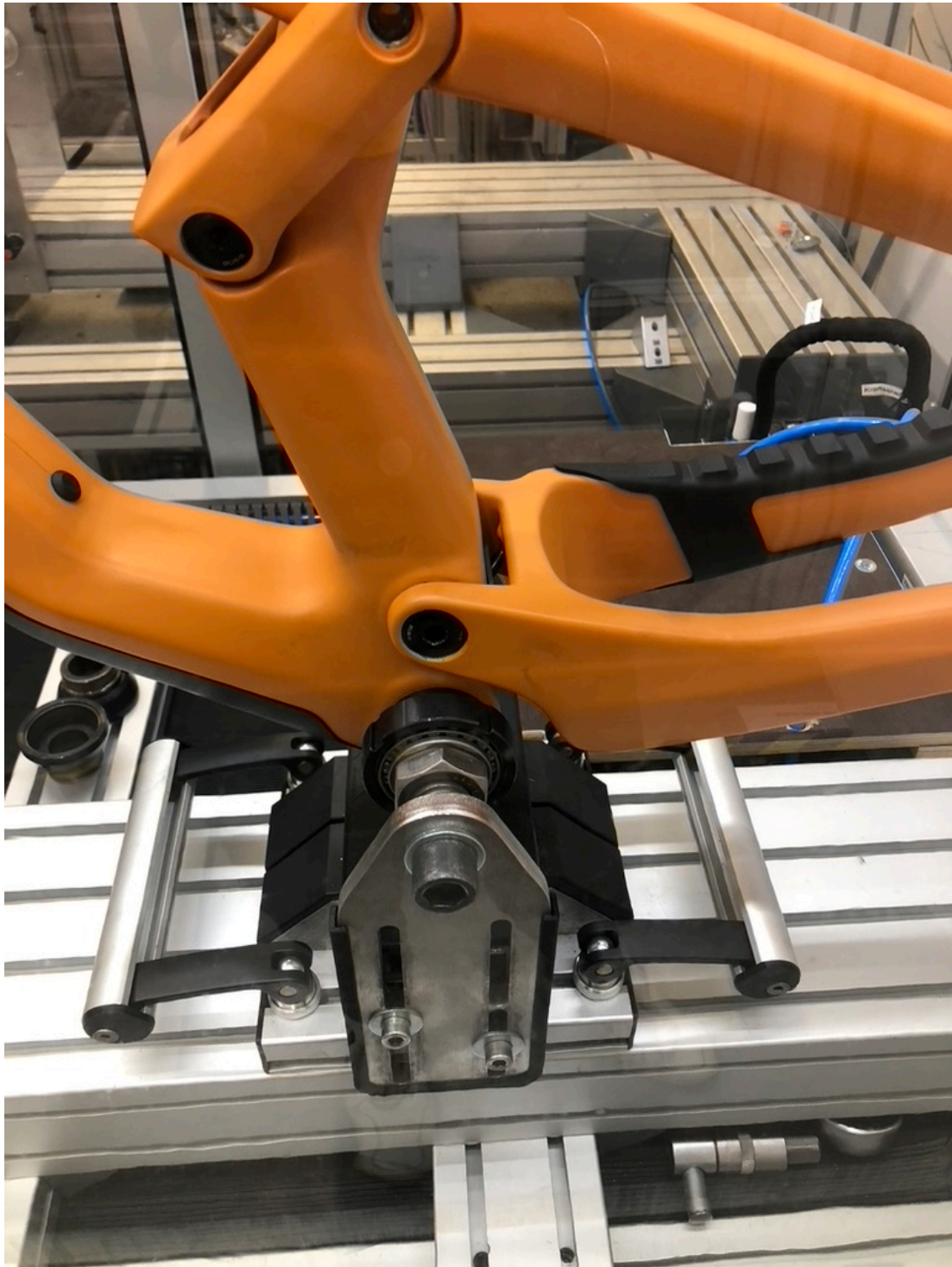
Figure 57 Bottom bracket fixture in the scrub load fatigue test bench.
