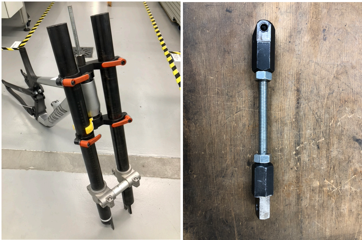
Figure 4 Examples of Canyon's fork and shock dummies.
