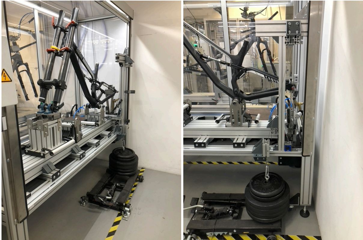
Figure 69 Final test setup of the angled force.
