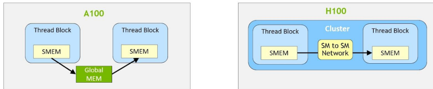
Figure 2.4: Comparison between traditional thread-block data exchange through global memory on A100 and cluster-level data exchange through distributed shared memory (DSM) on H100 [9].
