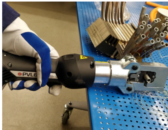
Figure 12.3: Crimping the junctions.
