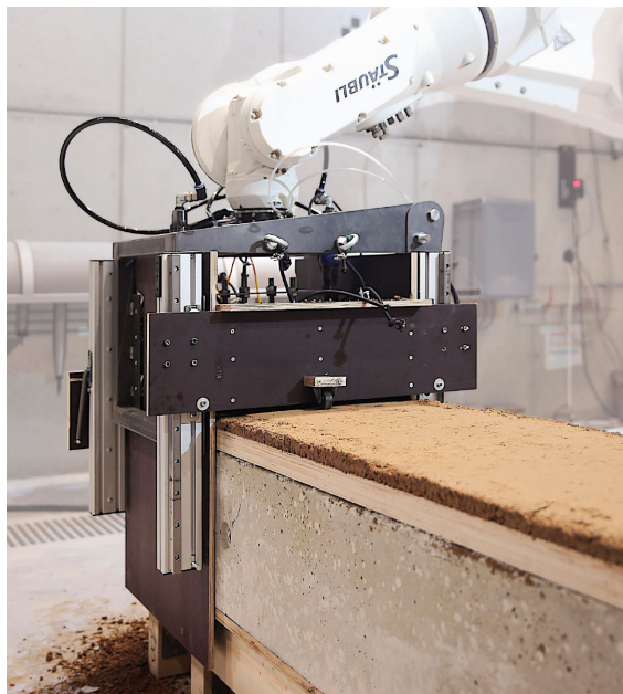
Figure 18. Robotic fabrication of rammed earth elements - Digital Building Fabrication Laboratory (DBFL) at TU Braunschweig. Photo ITE/TU Braunschweig
