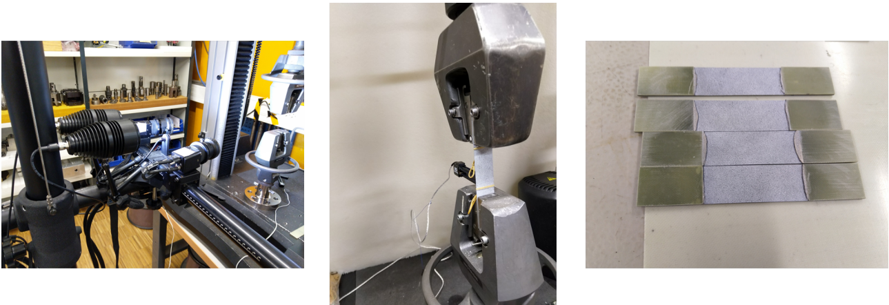
Figure 3.5: The left picture shows the DIC-cameras mounted in front of the tensile test machine, in the middle picture is a specimen clamped in the tensile test machine and the right picture depicts four tabbed specimens ready for testing.
