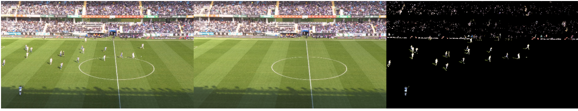
Figure 4.6: Foreground extraction. The leftmost image displays the original frame, the middle image illustrates the background after extraction, and the rightmost image shows the foreground with the moving objects clearly isolated.
