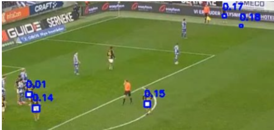
Figure 4.5: YOLOv9 detection boxes with confidence scores, identifying players' white shorts, and text in the background, as balls.
