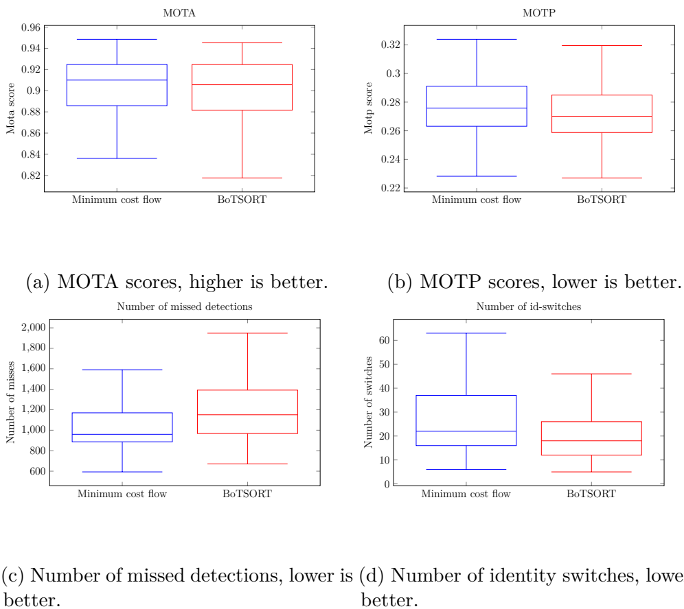
Figure 4.9: Comparison of MCF and BoT-SORT algorithms in various metrics, showing similar performance.
