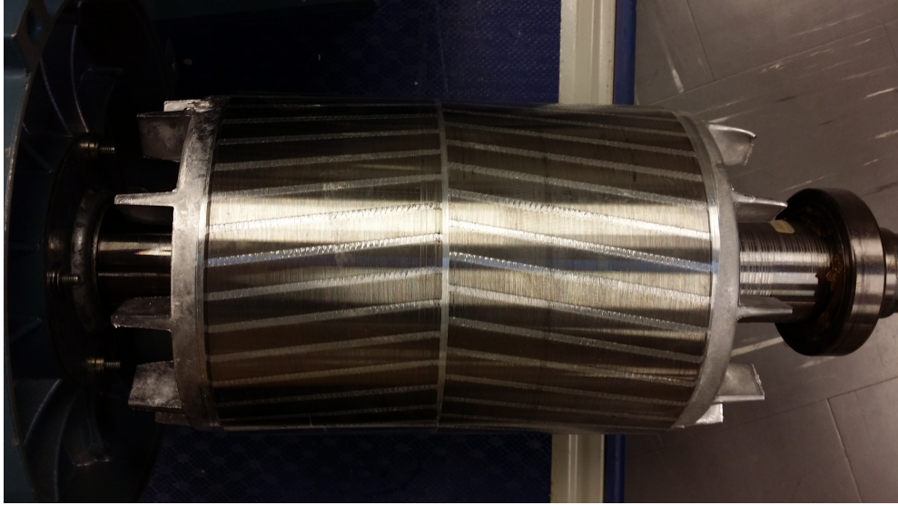
Figure 2.1: Example of a skewed rotor.
