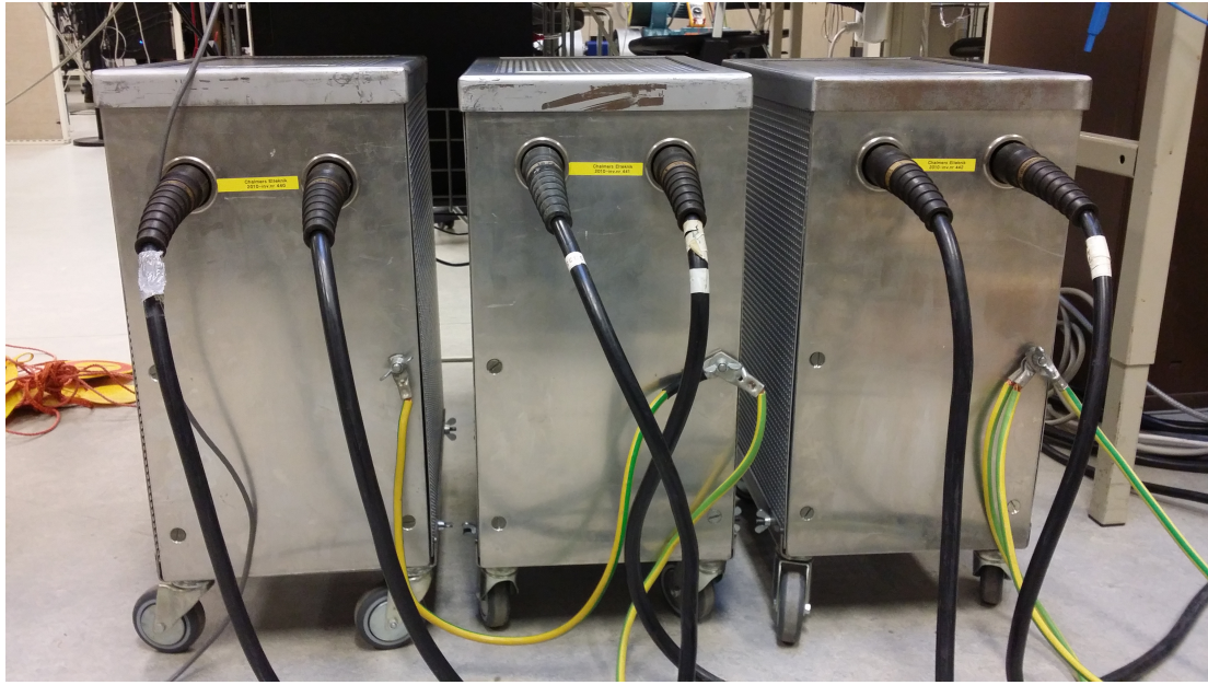
Figure 3.5: Resistors used for the tests connected on series between generator and machine.
