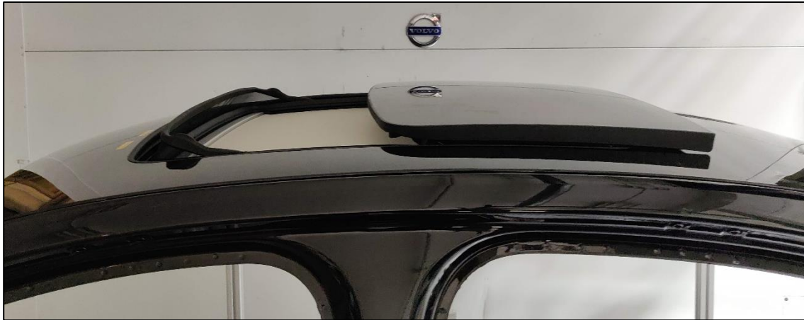
Figure 29 Sunroof panel in its fully open position
