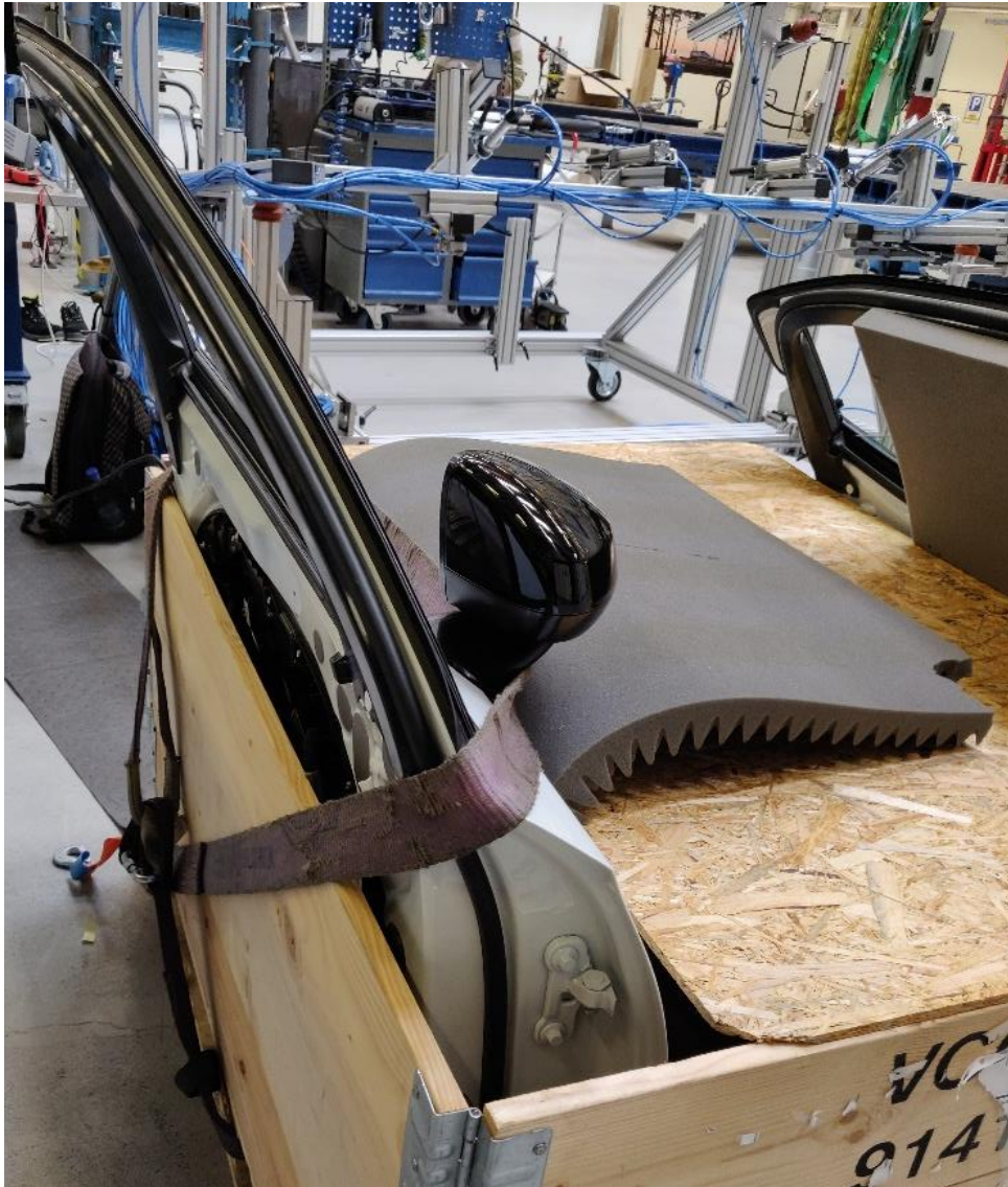
Figure 59 One of the attempts of securing the front door in one position so that reliable measurements could be taken without that the door moved
