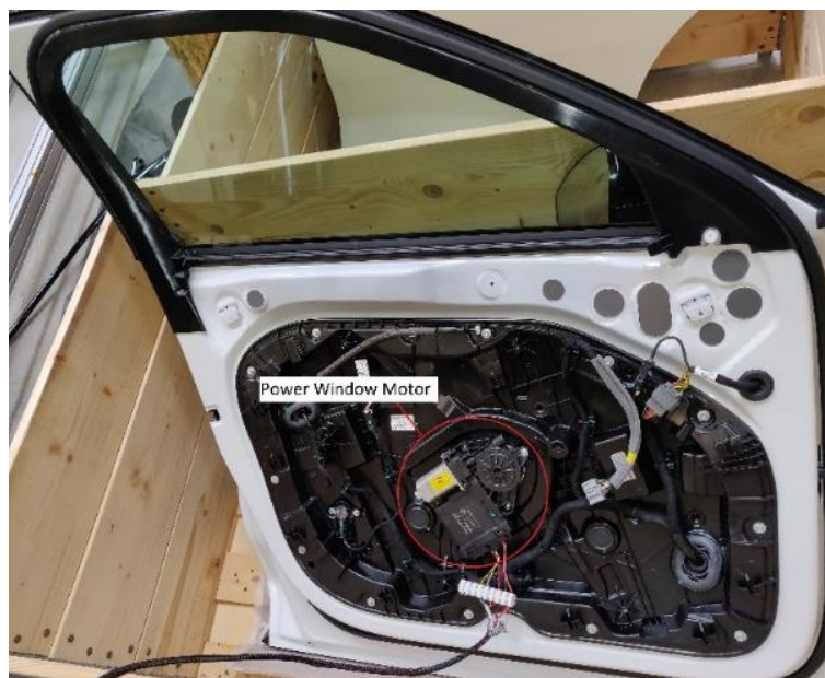
Figure 22 Inside of the front door showing the placement of the power window motor
