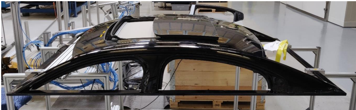
Figure 18 The cut off section of the roof, including sunroof panel and curtain mounted on a trolley
