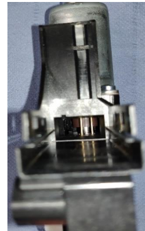
Figure 24 The opening in the motor where the hall sensors are inserted
