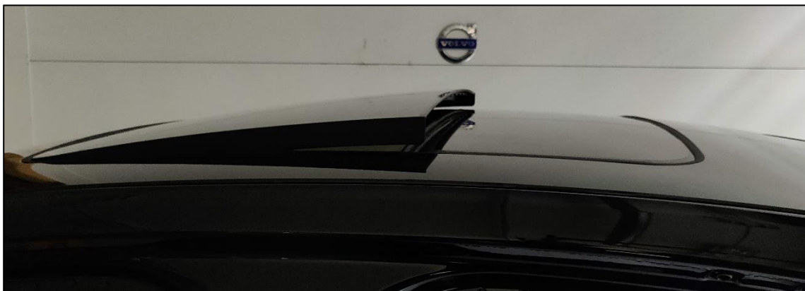
Figure 28 Sunroof panel in its tilted position
