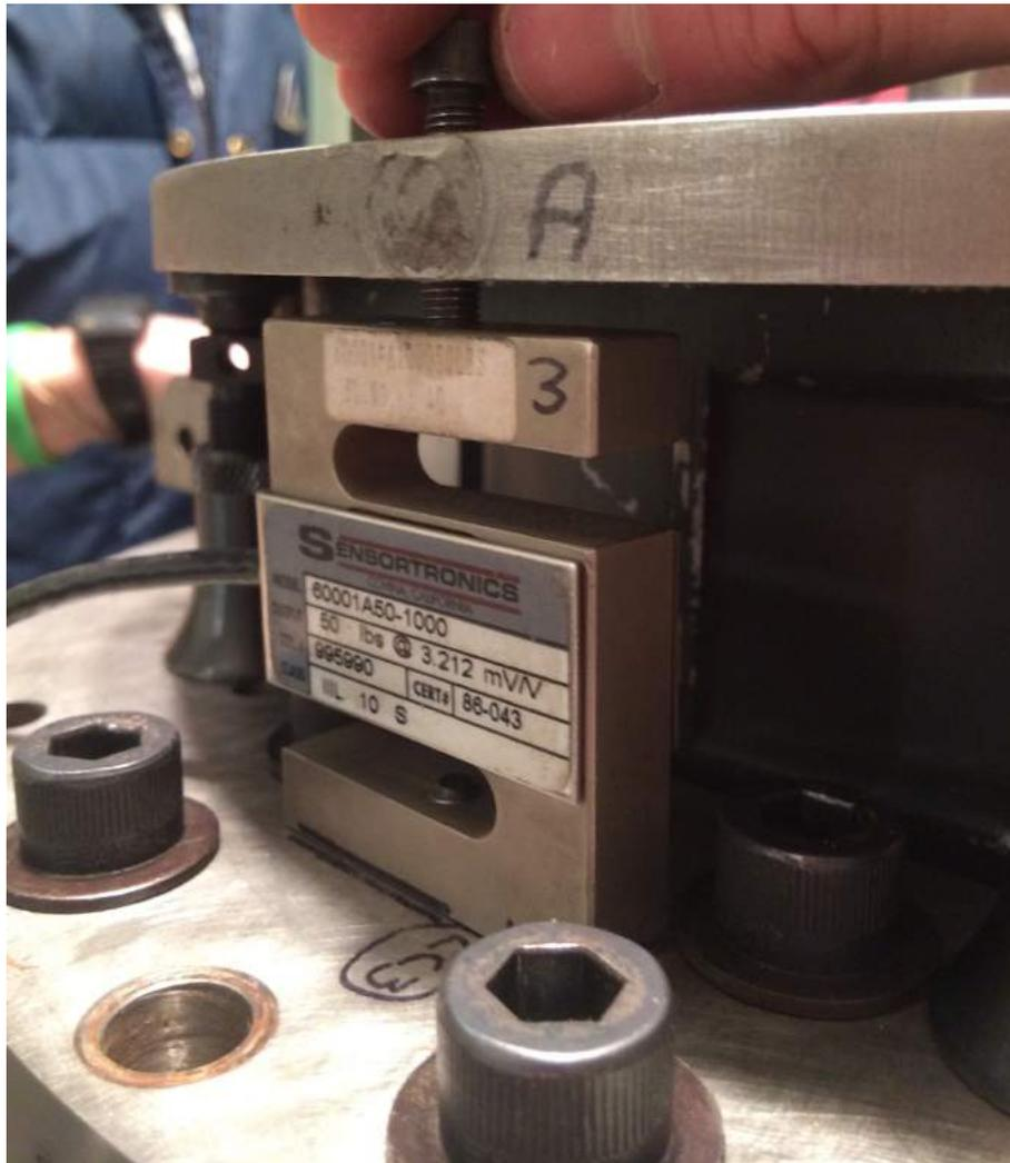
Figure 4.8: Mounting load cells to the motor hub.
