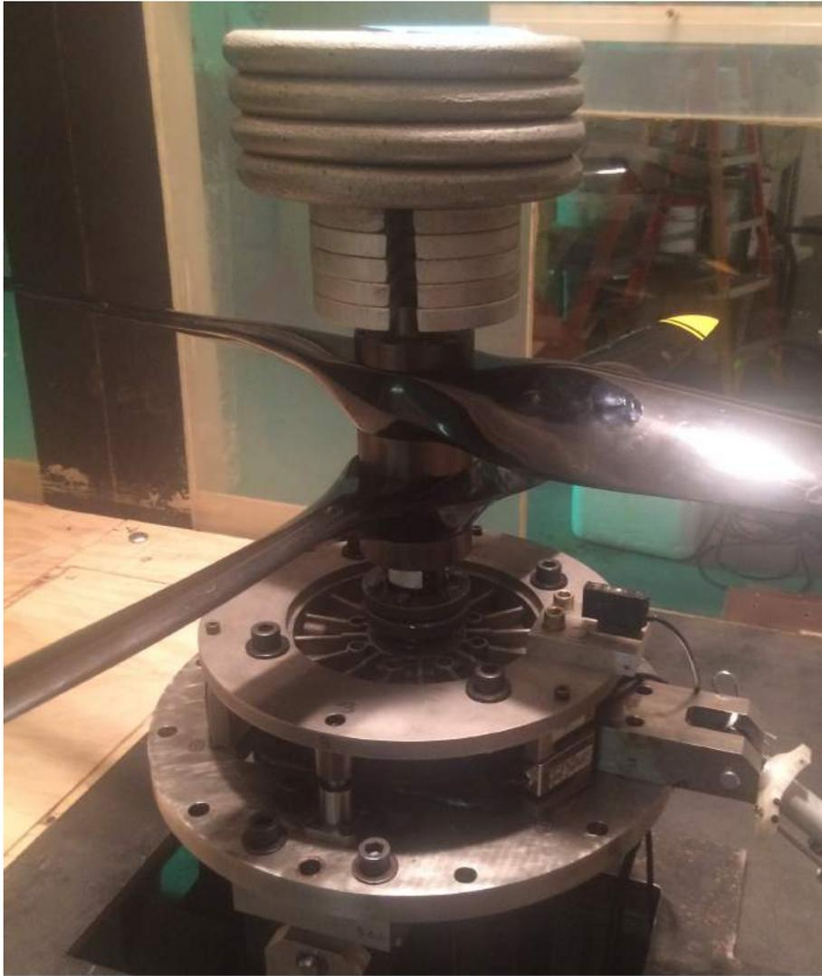
**Figure 5.1:** 50 pounds in load stacked on the hub
